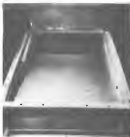
Figure 5. Filter layer after backflushing
