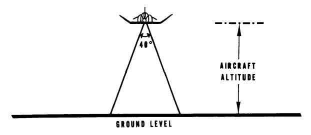
The IRLS is a cryogenic device (optical and electronic) capable of detecting passive electromagnetic energy resulting from target thermal emissions in the infrared band from 8 to 14 microns (1 micron= $10^{-6}$  meters). It has a cross-track scan angle of  $120^{\circ}$  about the aircraft's nadir, as shown below:
