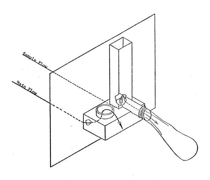
Figure 1. Plan view of proportional sampler.
