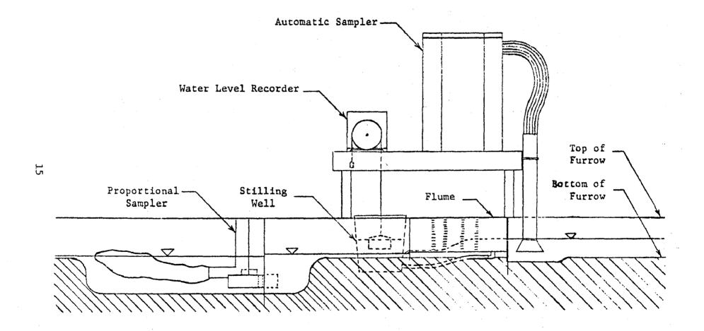
Figure 2. Field installation of proportional sampler and flume-recorder-sampler setup.
