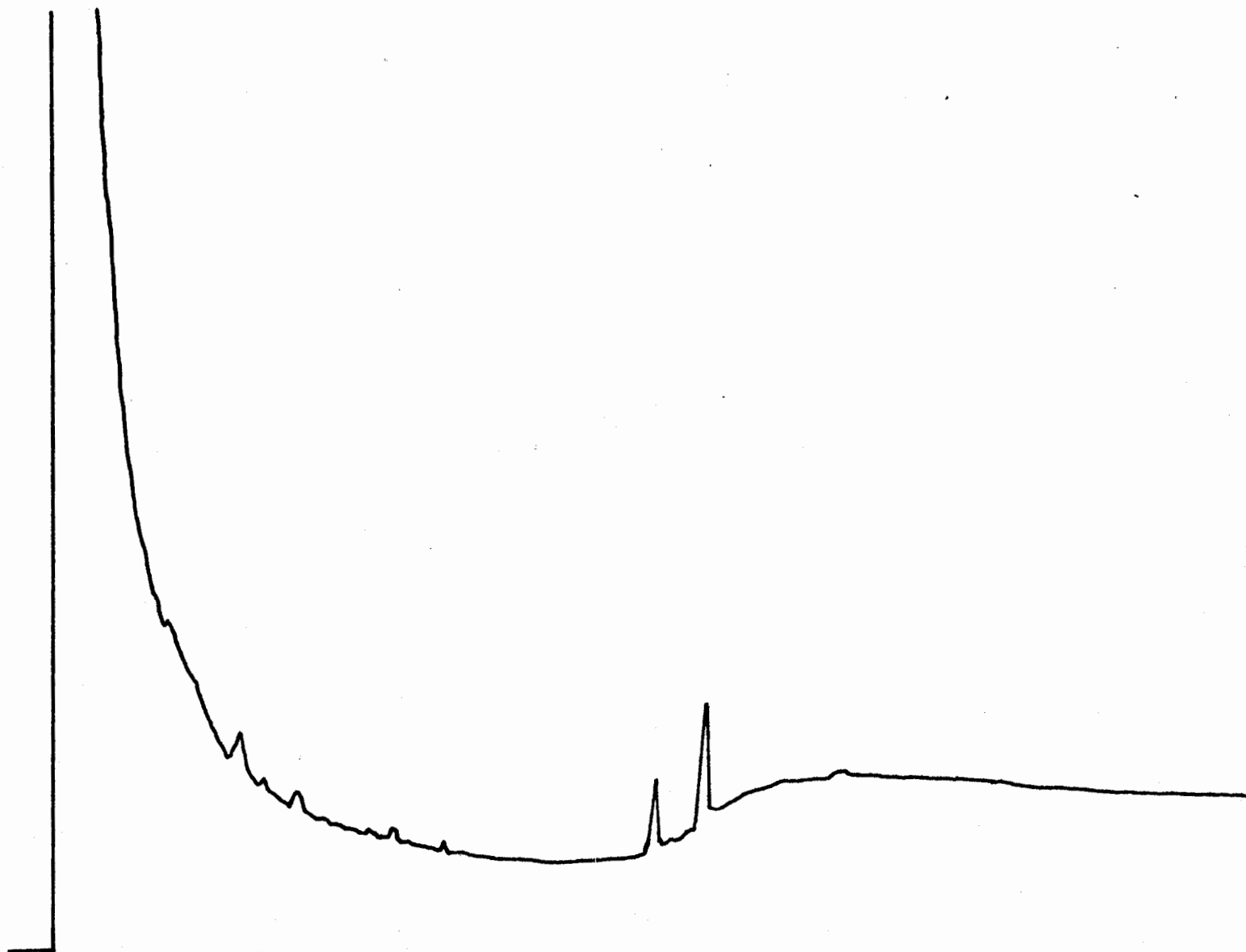
Figure B-1. FID chromatogram of Lake Superior sediment extract after clean-up by florisil column chromatography, gel permeation chromatography, and silica gel column chromatography (benzene eluate).
