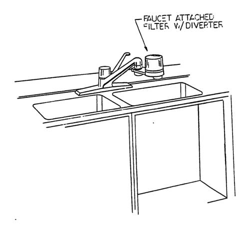
Figure 1. Schematic diagram of faucet filter as it is installed (courtesy of P. Regunathan).
