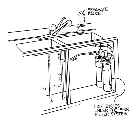
Figure 2. Schematic diagram of bypass filter as it is installed (courtesy of P. Regunathan).
