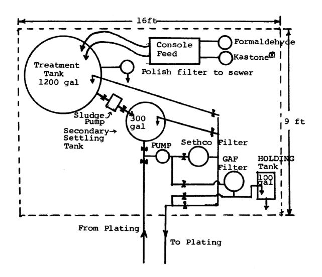
Figure 3. Approximate positions of current equipment and over all area. No attempt has been made to exact scale each item. This figure merely shows the juxtapositioning of the various elements and the plumbing to each.
