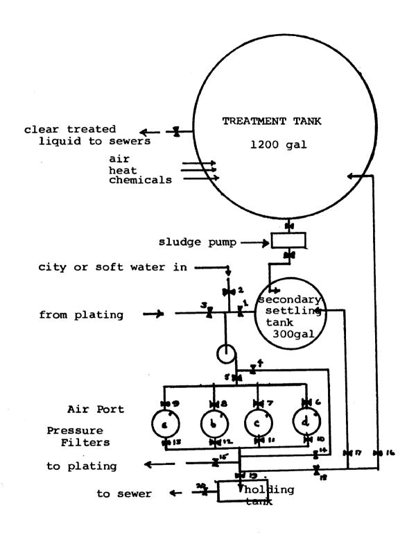
Figure 1 Proposed Treatment and Recycling System.
