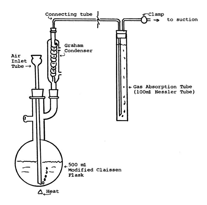
Figure 4. Total distillation apparatus
