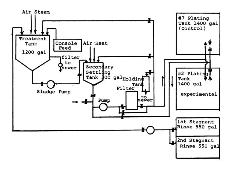
Figure 2. General layout of treatment and recycling equipment.
