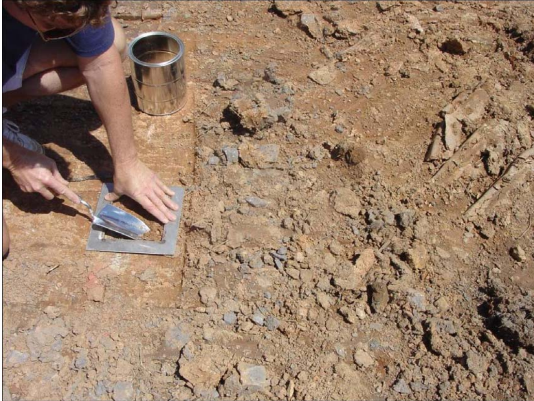
Figure 5-1. Soil sampling after the NESHAP demolition.
