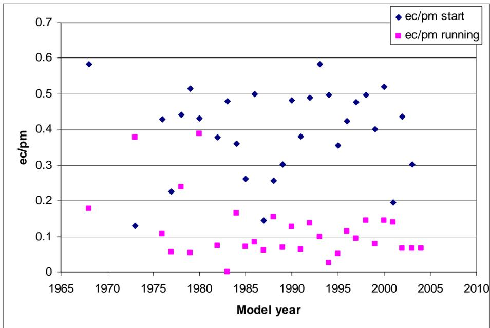
**Figure 43. Elemental Carbon to Total PM ratio as a function of vehicle model year.**
