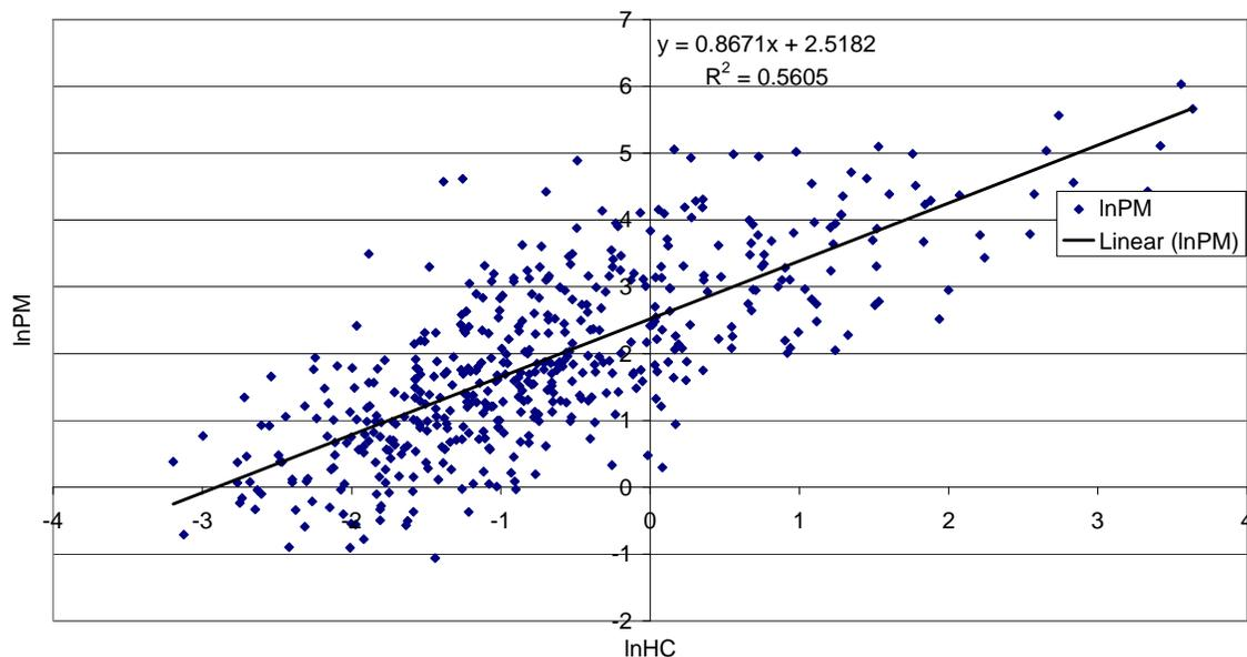
Figure 23. PM correlation with HC (not temperature adjusted).
