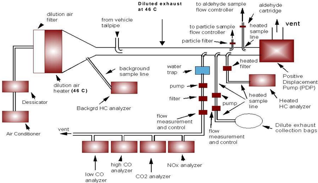
**Figure 3. CVS Sampling System Schematic**
