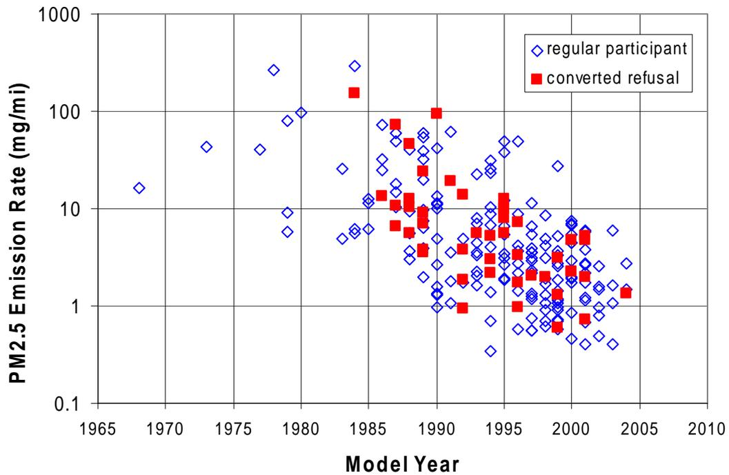
Figure 5. Aggregated PM Emissions in Round 1 (logarithmic scale).
