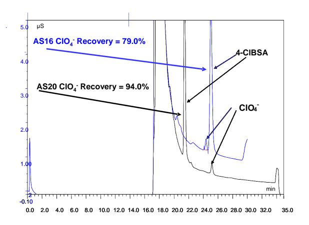
Figure 2  $IC\ CHROMATOGRAM\ of\ SURFACE\ and\ GROUND\ WATER$  FORTIFIED WITH 1.0  $\mu g/L\ ClO_4^-$
