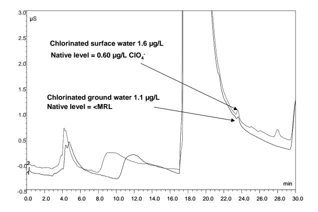
Figure 3  $IC~CHROMATOGRAM~of~3.0~\mu g/L~ClO_4^- in~50,~500~and~1000~mg/L~LSSM~WITH~the~IONPAC~AS16~COLUMN$
