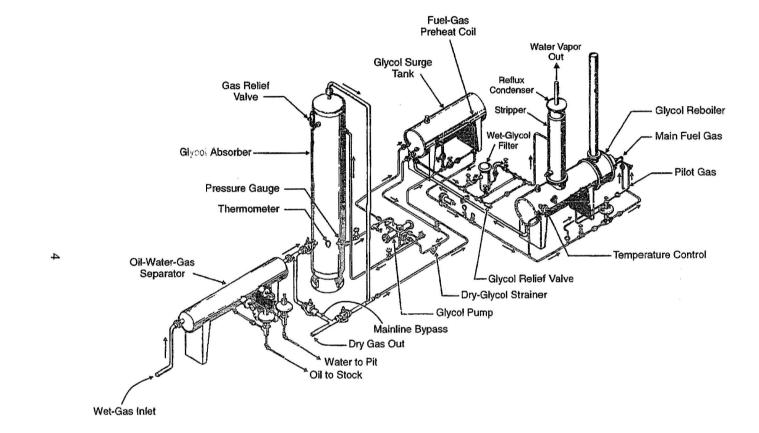
Figure 3-1. Isometric Flow Diagram of a Glycol Dehydrator Unit
