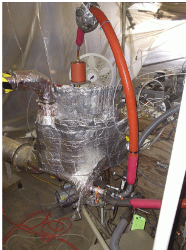
Heated lines attached to probes into CVS tunnel
