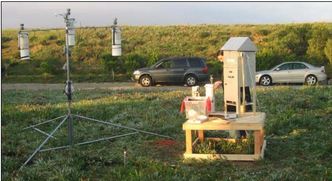
Figure 2-3. MiniVol (three) and HiVol instrumentation as deployed at the East Tarmac during a portion of the winter monitoring program.
