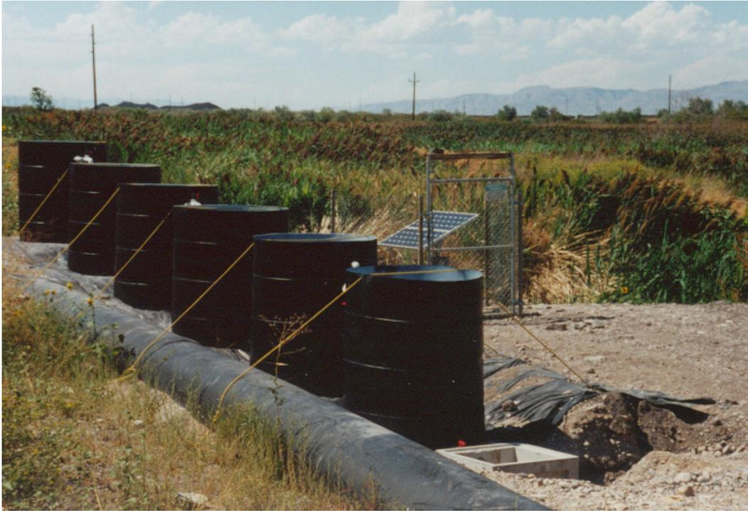
**Figure 1-7. Field-scale BSeR™ process reactor.**
