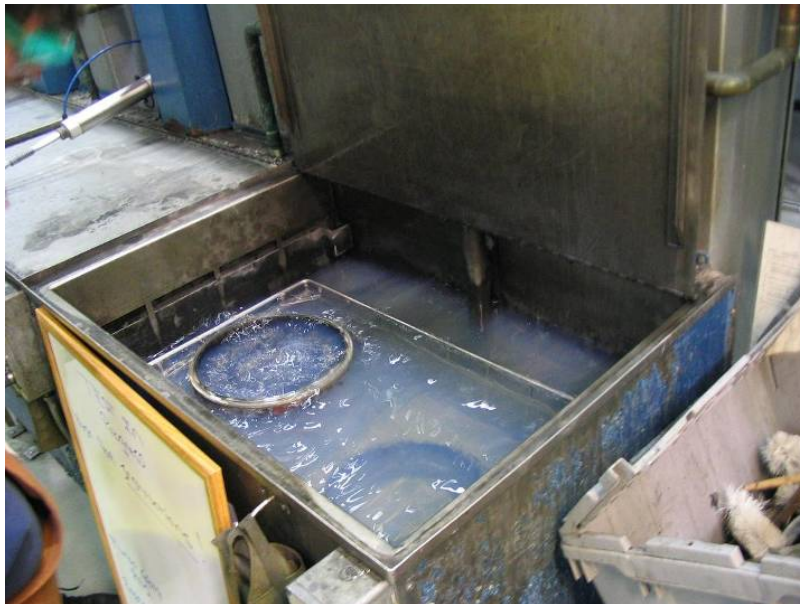
Figure 10. Eagle Kleen™ Degreaser Bath
