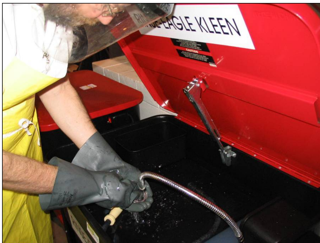
Figure 6. Wheel Bearings Being Degreased with Eagle Kleen™
