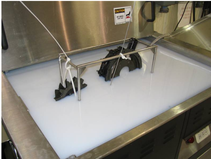
Figure 17. Parts Partially Suspended in Cleaning Bath
