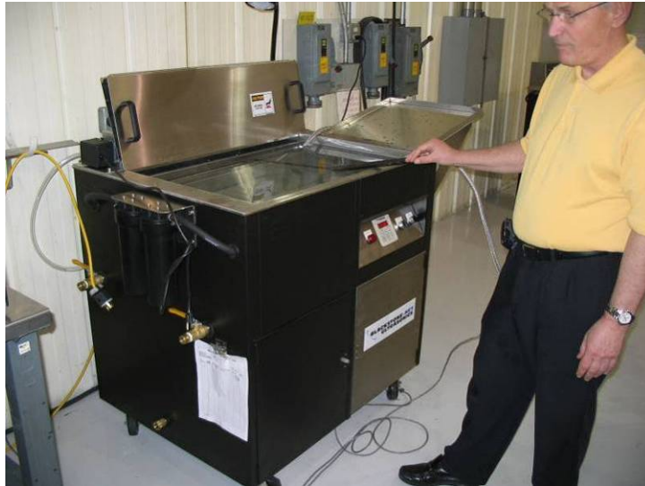
Figure 15. “Grease Monkey” CLASSIC 3523 Blackstone~Ney Parts Washer
