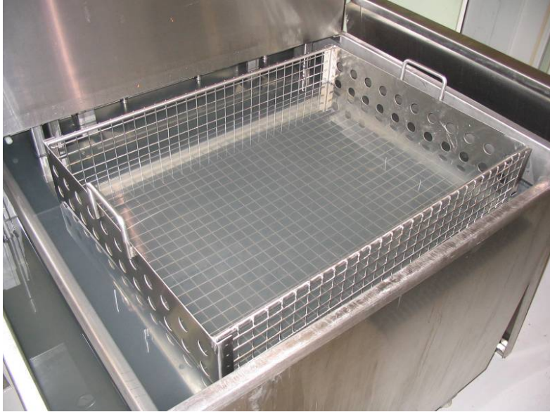
Figure 22. Agisonic AG-30 Looking Down into Basket (Note: the tray is in the parts-loading position)
