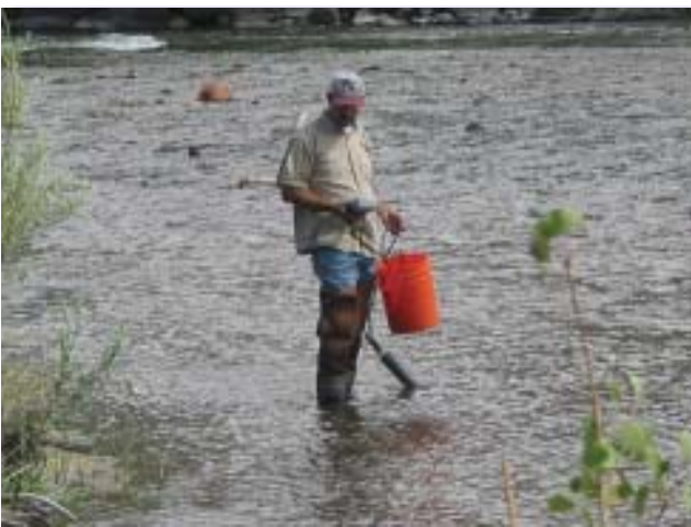
Monitoring with a YSI sonde on the Truckee River.
