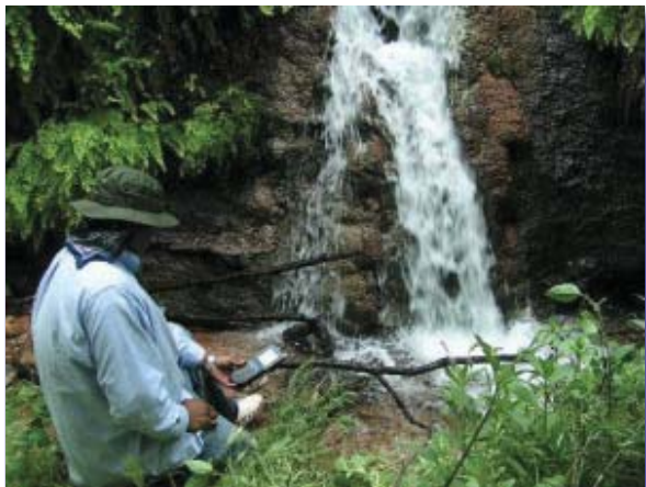
Sampling basic water quality parameters just below Diamond Spring by Anthony Raymond, Water Resources Technician.
