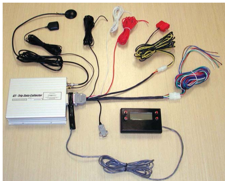
Figure 1: Configuration of the Georgia Tech Trip Data Collector
