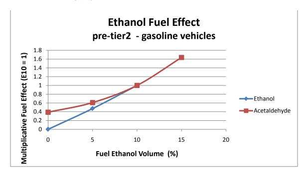
Figure 10-5 shows the relationship between fuel ethanol and exhaust ethanol and acetaldehyde emissions. These are shown on a separate figure because the fuel effects range from zero to almost a factor of two for these two air toxic pollutants. Both these curves show a strong and predictable response to fuel ethanol from 0 to 10 percent ethanol.
