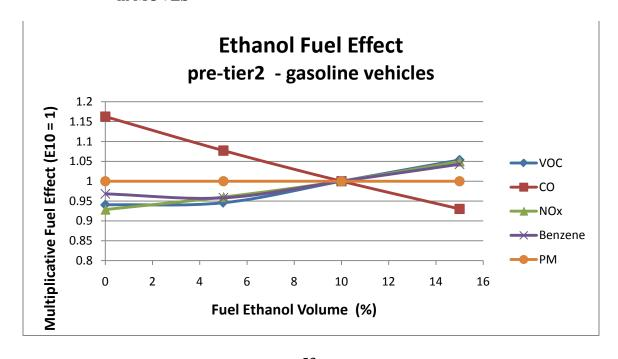
Figure 10-5 Relative Fuel Ethanol Effect on Pre-2004 Model Year Gasoline Vehicles in MOVES
