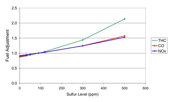
Figure 10-3 Relative Fuel Sulfur Effect on 1988 Model Year Gasoline Vehicles in MOVES
