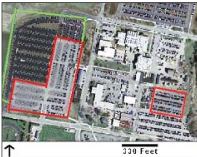
URI's permeable parking lots - The two original permeable asphalt parking lots built in 2002 and 2003 are outlined in red. The 2005 parking lot extension is outlined in green.
