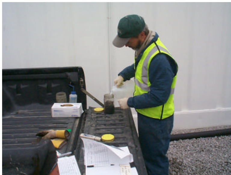
Photo 7: Leachate pH/Temperature /Conductance Sampling Using a Bench Top AccuMet AR20 Instrument
