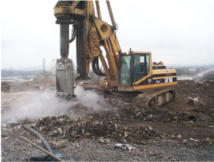
Photo 3: Fresh Waste Sample Collected from Drill Rig Using a 3-foot Bucket Auger
