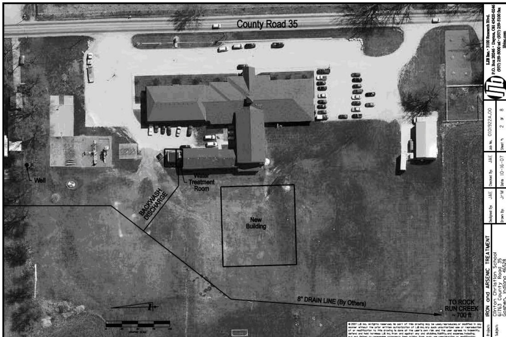
Figure 4-12. Layout of Backwash Discharge Drain Line at Clinton Christian School (LJB Inc., 2007)
