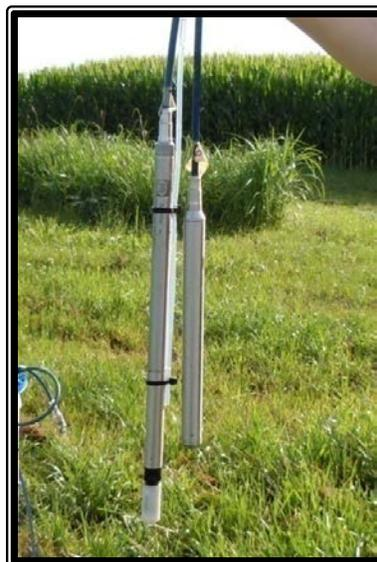
**Figure 3-4. Nitrate Sensor with attached Conventional Sample Tubing**
