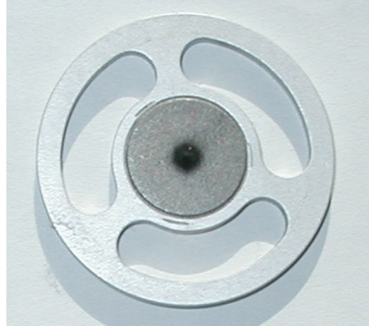
Figure 2-6. Coarse Urban PM (Diameter > 2.5 microns) with a Black Surface Coating, shown on a Filter from a Harvard Impactor Run Approximately 100 feet Above Street Level in Boston. (Photo courtesy of NESCAUM)
