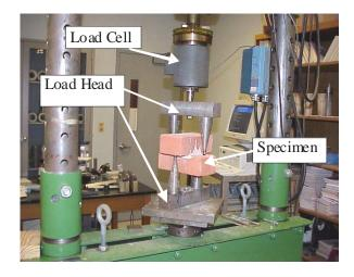
(a) Test specimen configuration
