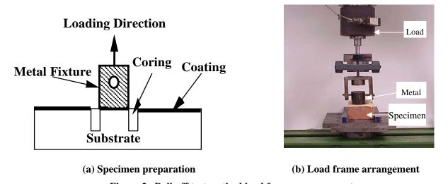
Figure 2. Pull-off test method load frame arrangement.
