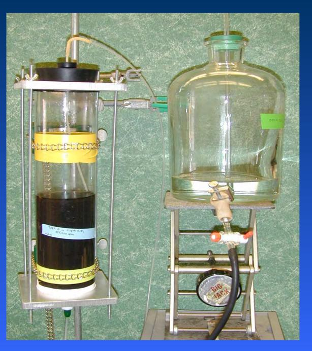
Glass column packed with Silt Loam Soil or Sand
