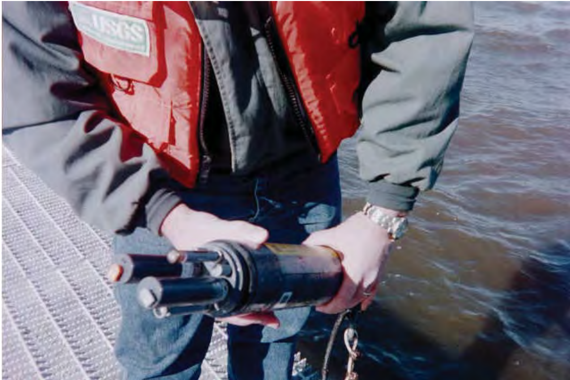
Figure 3.5. Picture of the YSI 6600 sensor package with multisensor probes taken during the January 9, 2001 site visit.
