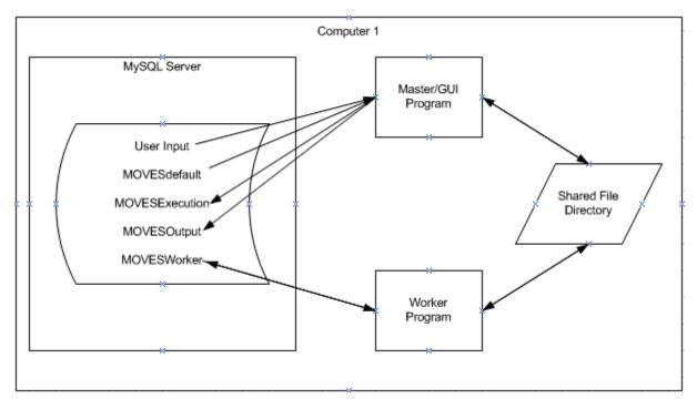
MOVES may also be configured so that several computers work together to execute model simulation runs. This can significantly improve execution time performance of large simulations. Improvements diminish, however, as more worker computers are added. The number of worker computers needed to approach the minimal execution time for a model run depends on the specific nature of the run.
