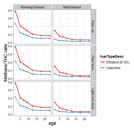
Figure 3-2. Methane/THC ratios by age, and source type for Gasoline and Ethanol (E85) fueled vehicles in model year 2005 and later
