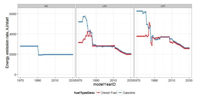
Figure 2-4. Cold start energy rates (opMode 108) for motorcycle, light-duty vehicles, and light-duty trucks
