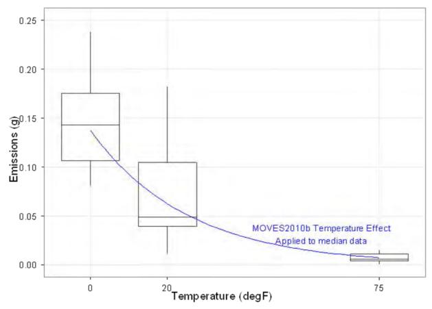
Figure 2-8 graphs the light-duty multiplicative temperature effects using the coefficient in Table 2-10, and the model form of Equation 2-9.
