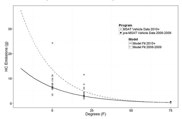
Figure 2-2 FTP HC start emissions with log-linear model fit
