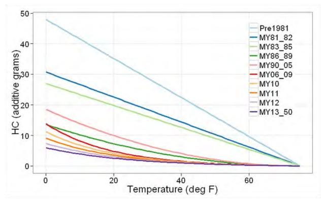
Figure 2-4 HC additive cold start temperature effects for gasoline vehicles by model year groups
