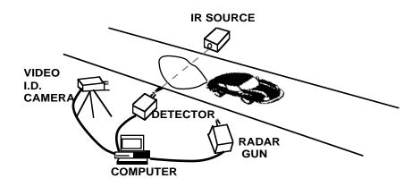
As a vehicle passes through the beam, the device measures the ratio of CO (and exhaust HC) to carbon dioxide in front of the vehicle and in the exhaust plume behind. The system uses the "before" measurement as a base and calculates the vehicle's CO emission rate by comparing the "behind" measurement to the expected ratio for ideal combustion.
