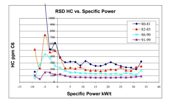
Figure 5.2 RSD %HC (C6) vs VSP (Denver Remote Sensing Clean Screen Pilot 12/99)
