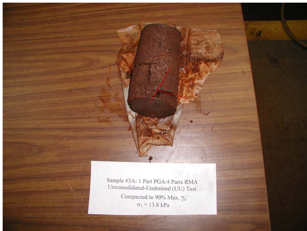
Mode of Failure
