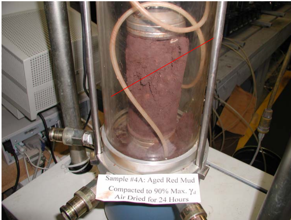
Mode of Failure
