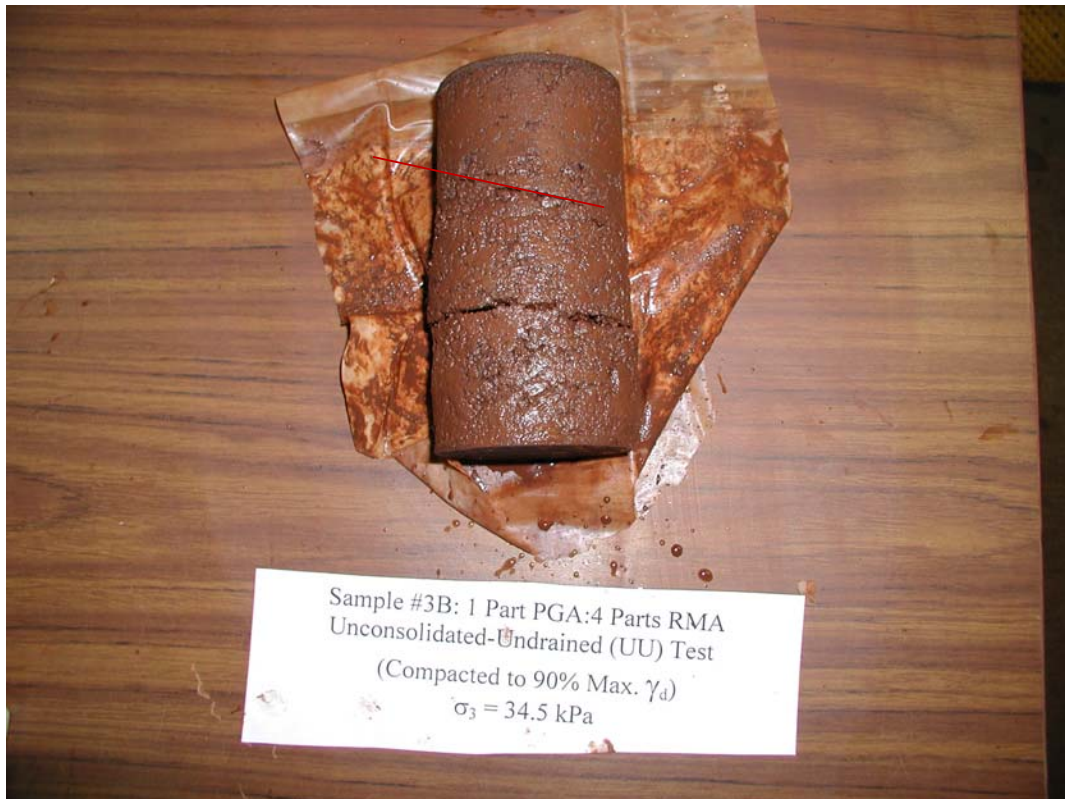
Mode of Failure
