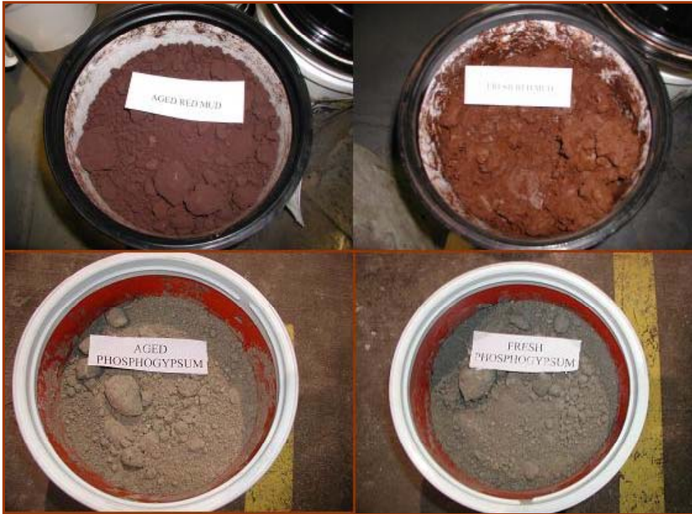
Figure 2-1. (a) aged red mud (top left), (b) fresh red mud (top right), (c) aged phosphogypsum (bottom left), (d) fresh phosphogypsum (bottom right)
