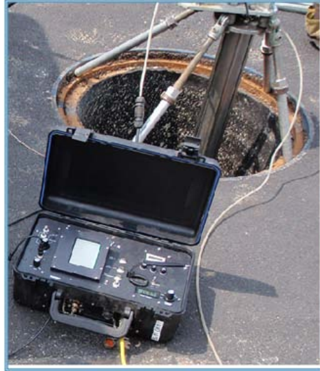
Acoustic unit recording reference sound signals at the insertion point.
