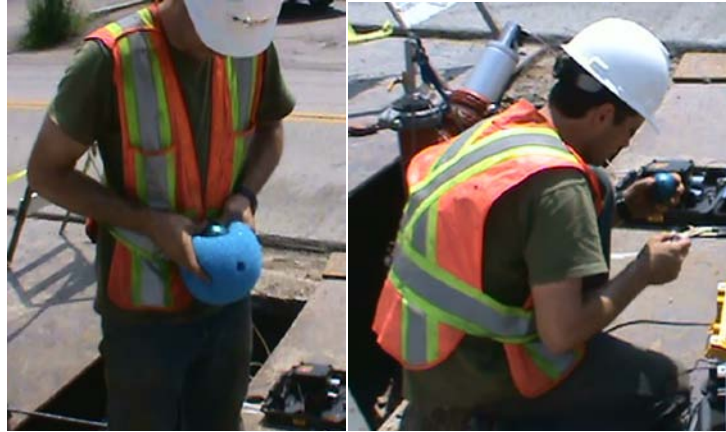
Figure 3-5. Aluminum Case and Foam Housing for SmartBall™ Acoustic Acquisition Device, Data Storage, and Power Supply
