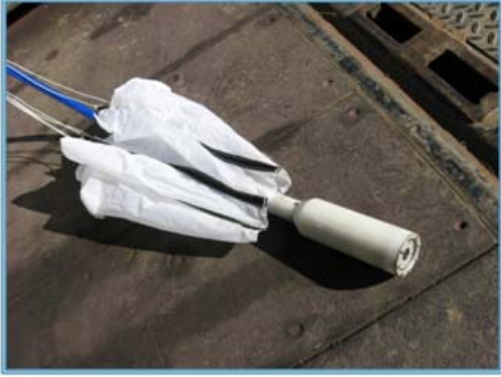
The Sahara Video sensor head and drogue.
