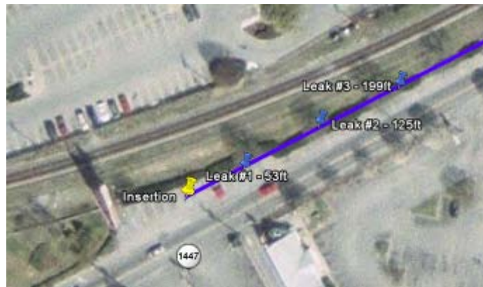
Figure 5.1c: Approximate Location of Leak
