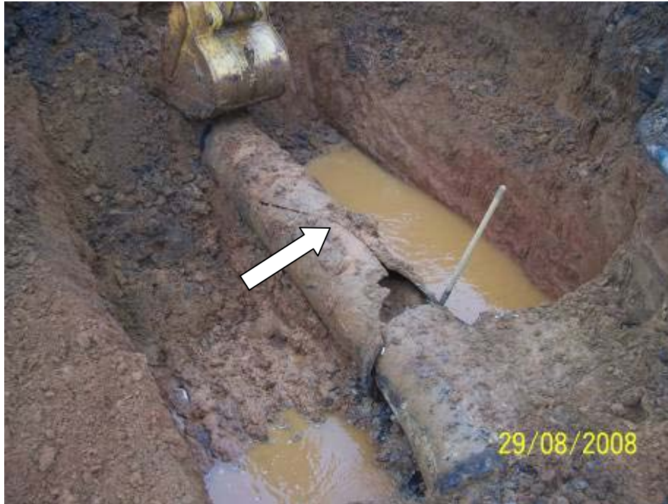
Figure 3-3. Pipe Break along Westport Road Adjacent to Test Area in August 2008
