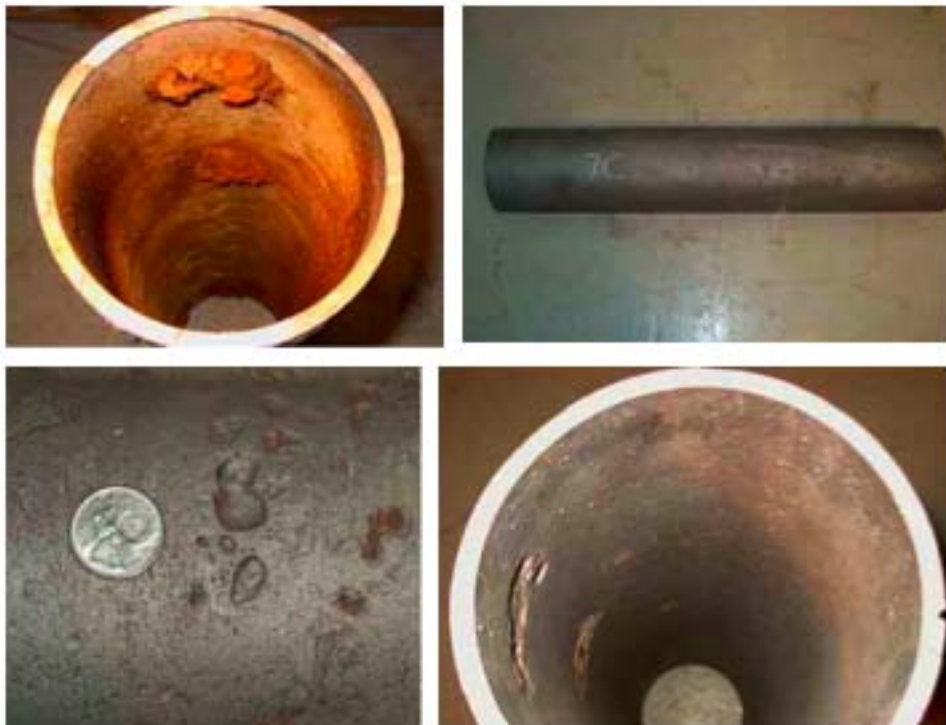
Figure 2: Photos of pipe with 8.9% measured loss
