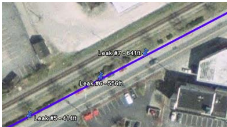
Figure 5.6c: Approximate Location of Leak
