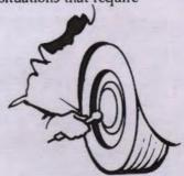
different inflation. You should check the pressure on all four tires every two weeks with an accurate hand-held air pressure gauge--service station built-in air pump gauges are sometimes inaccurate.
