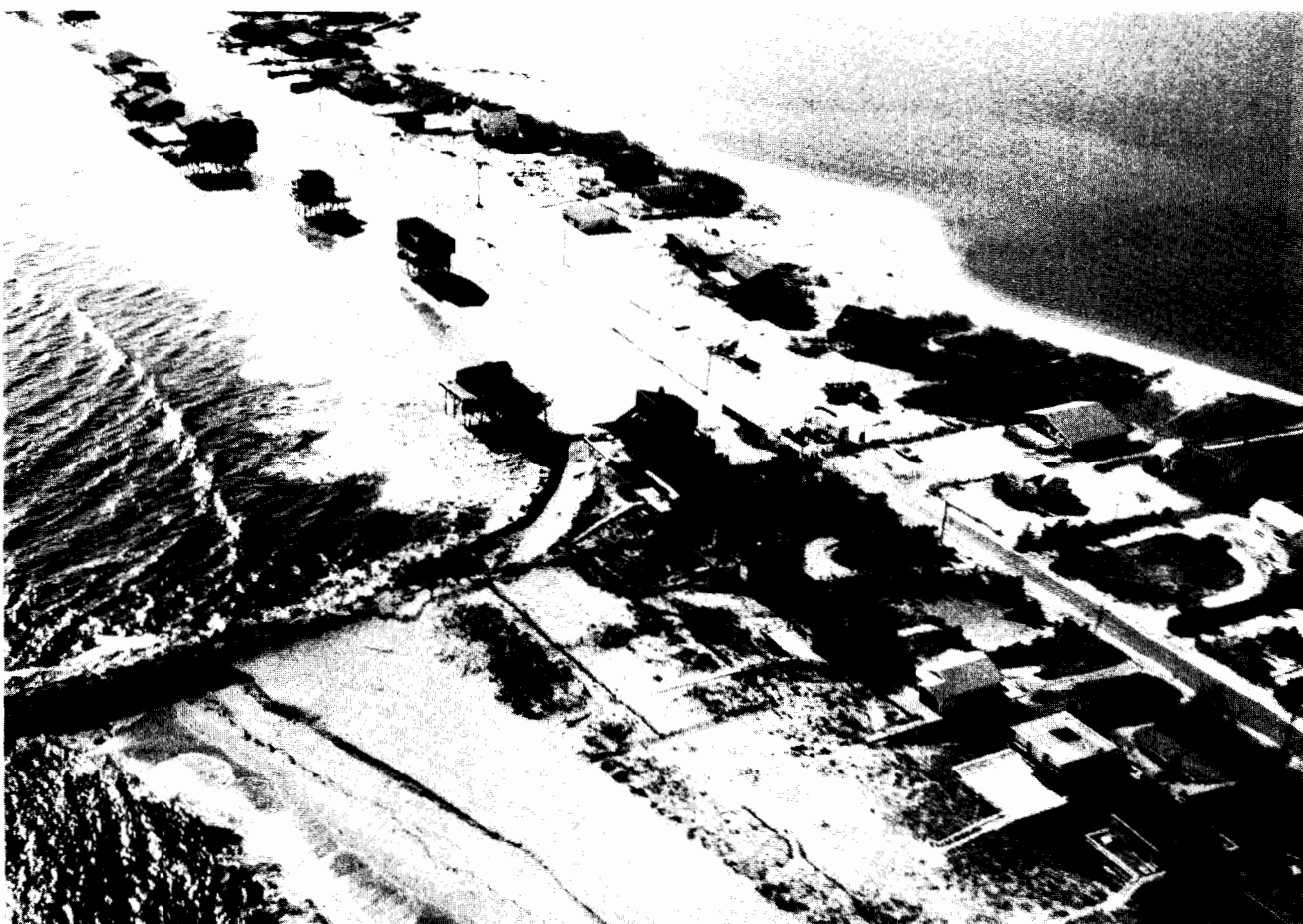
Figure 4. The effects of groins on the shoreline at Westhampton Beach, Long Island, New York, are obvious. While some property owners have greatly benefited from the emplacement of these shore-perpendicular structures, the downdrift beaches are quickly retreating and the sea is actively claiming residences.
