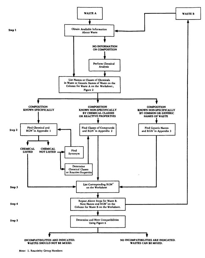
Figure 1. Flow diagram for determining hazardous waste compatibility.
