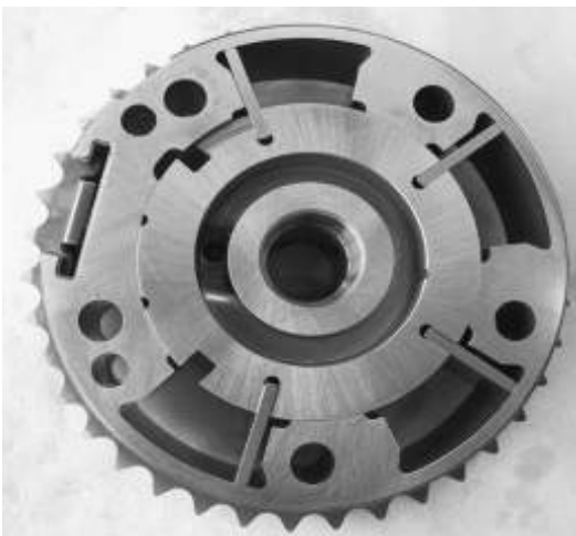
Figure 5-1: Hydraulic vane-type cam phaser
