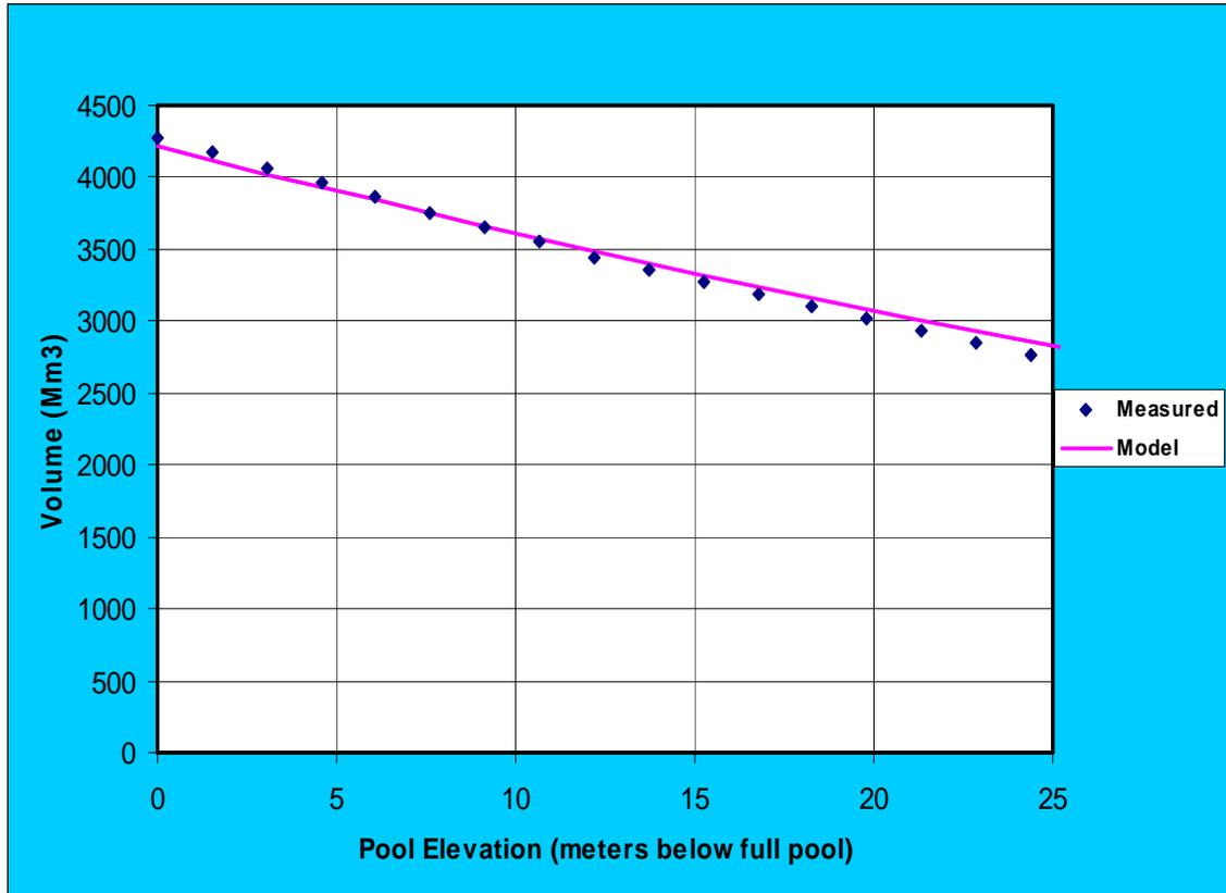
Figure 8. Modeled and observed reservoir volumes for Dworshak Reservoir
