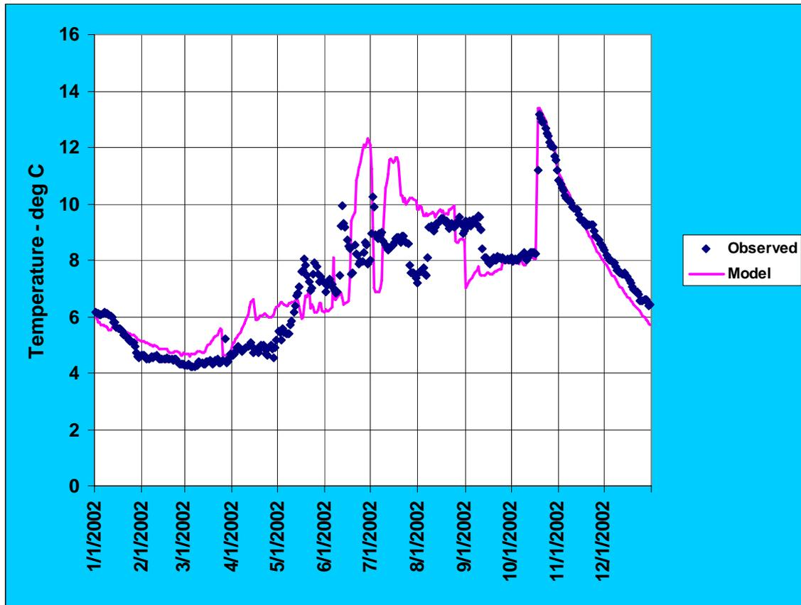
Figure 14. Simulated and observed outlet temperatures at Dworshak Dam during 2002.
