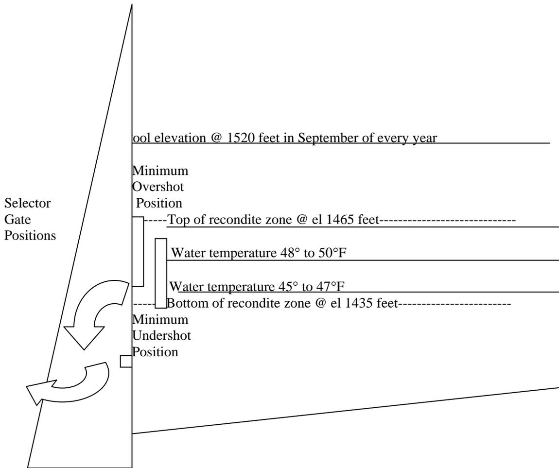
Figure 4. Dworshak Reservoir pool limitations in September
