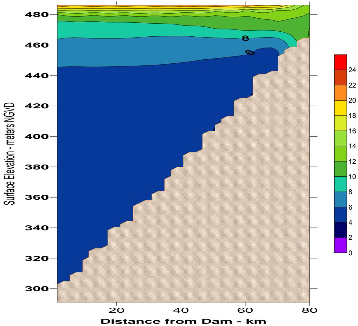
Figure 19. Simulated longitudinal temperature profiles in Dworshak Reservoir on June 30, 2002.
