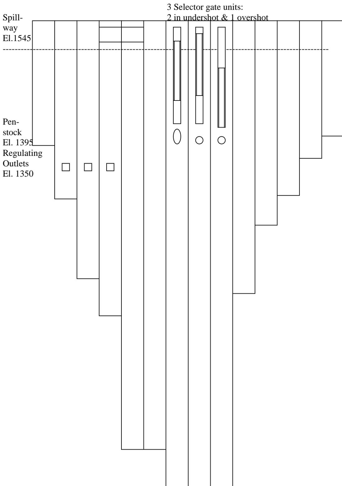
**Figure 2. Dworshak Dam face, looking from upstream to downstream**
