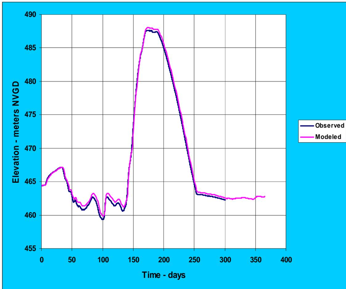
Figure 10. Measured and modeled pool elevation in Dworshak Reservoirs in 2002.
