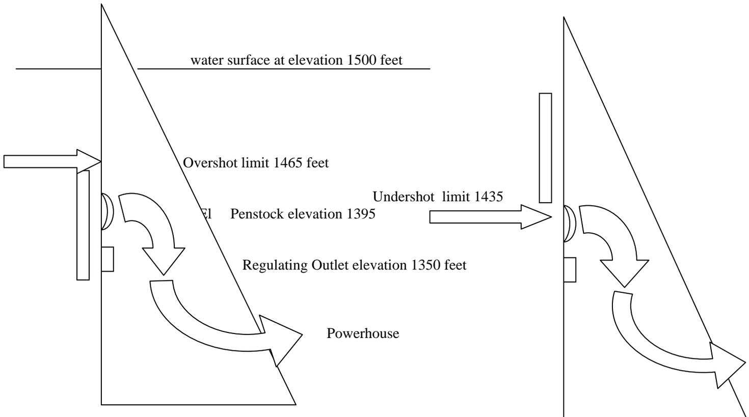
**Figure 3. Dworshak Dam selective withdrawal structure schematic**
