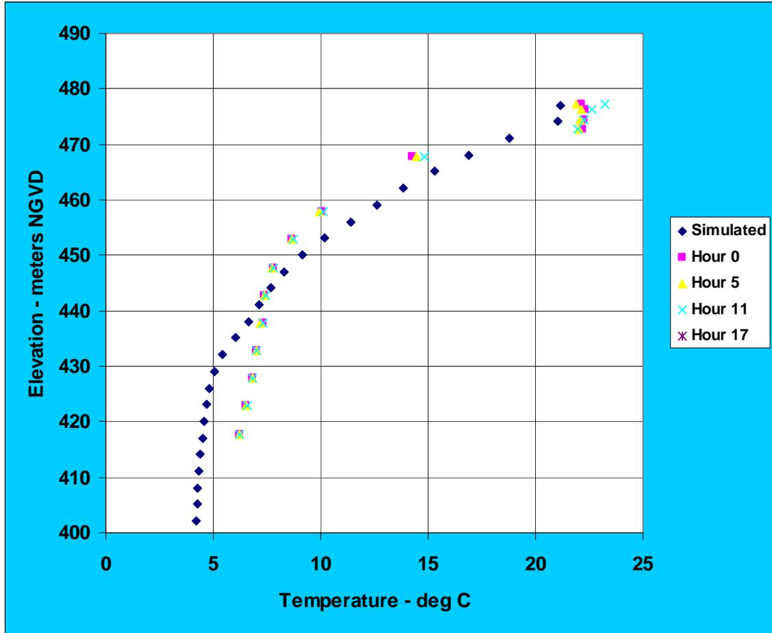
Figure 17. Simulated and observed water temperatures in Dworshak Reservoir at Dworshak Dam on August 8, 2002.
