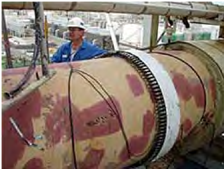
Figure A-6. The Teletest Remote Detection Tool Showing Transducer
