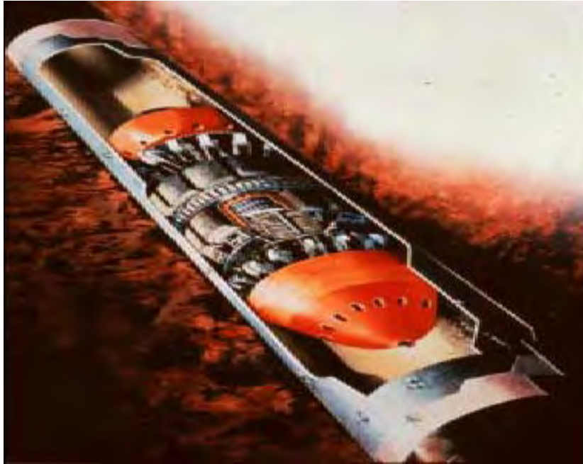
Figure A-8. An MFL In-Line Inspection Pig
