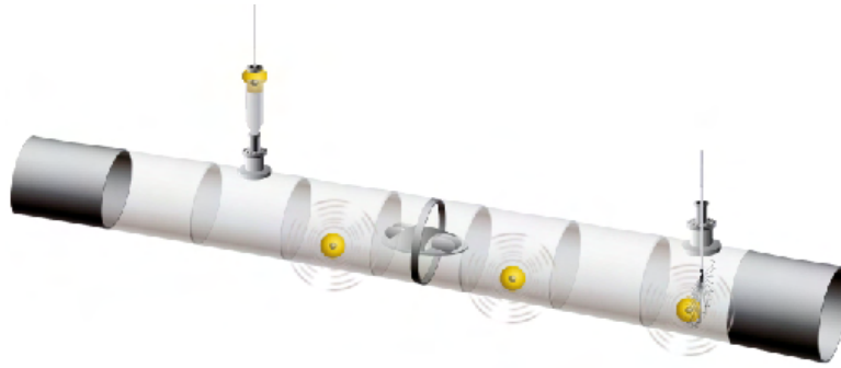
Figure A-21. SmartBall® Inspection Method – Insertion, Travelling, and Removal
