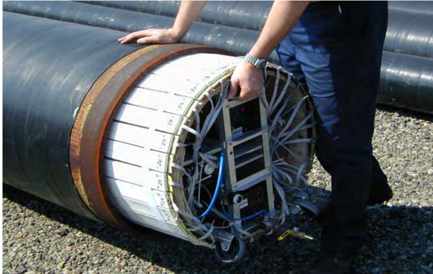
Figure A-13. A 24-in. BEM In-Line Intelligent Pig
