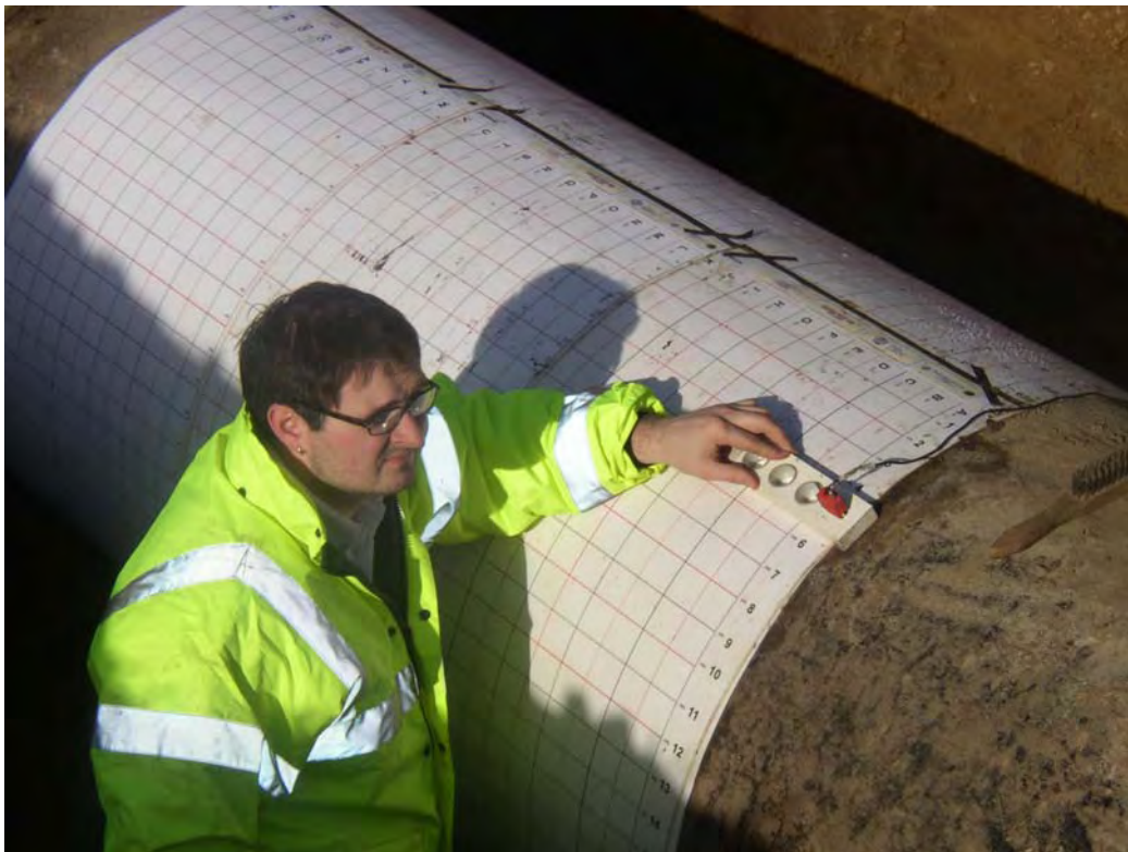
Figure A-12. A BEM Hand Held Tool Being Used to Scan a Gray Iron Pipe
