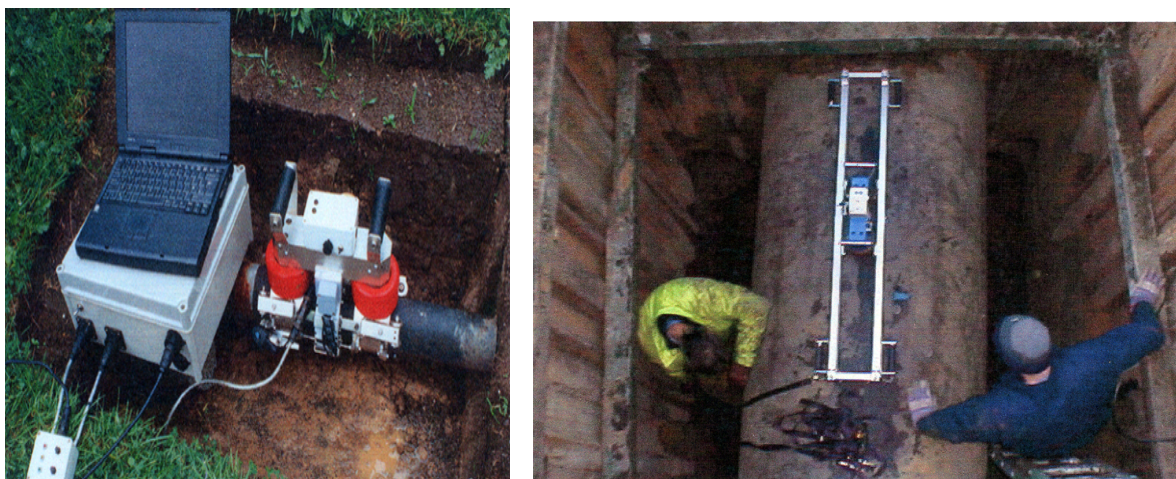
Figure A-7. AES S19 and AES ECAT Pipe Wall Inspection Tools
