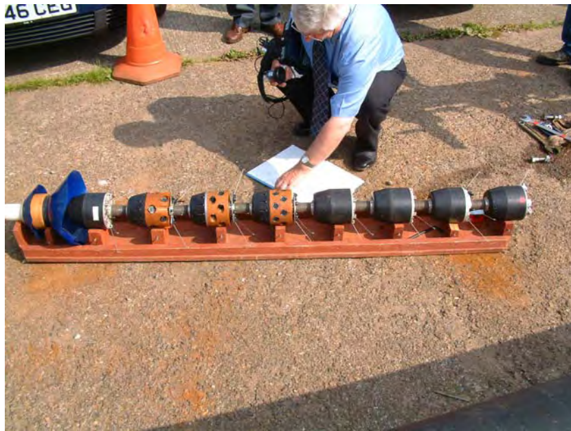
Figure A-16. Ultrasonic Super-pig Modules
