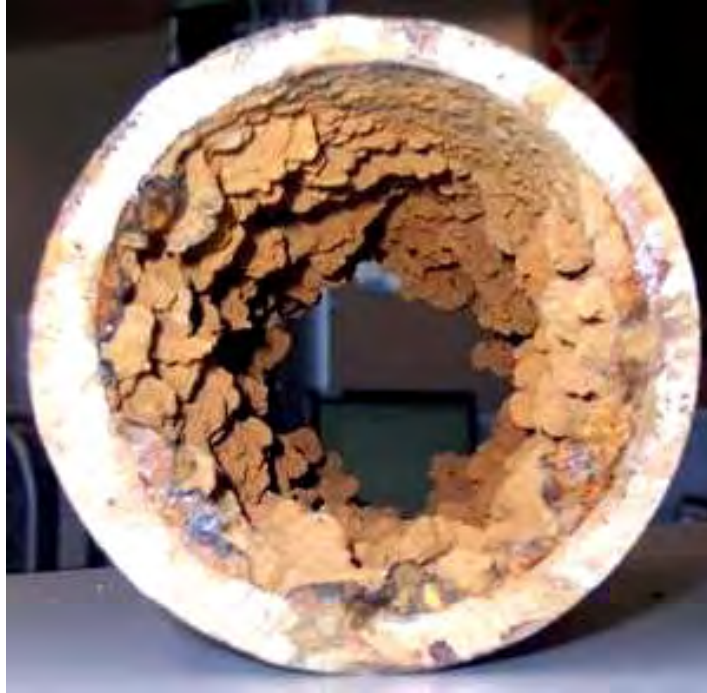
Figure 1-5. Tuberculated 6-in. Cast Iron Water Pipe
