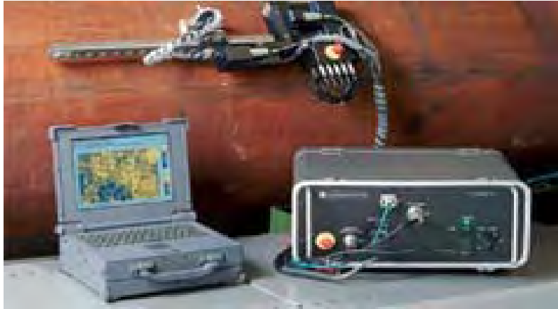
Figure A-2. IAS50 Ultrasonic Scanning Tool (GEI)
