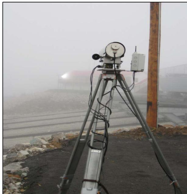
cannot identify specific compounds. One intended use of the instrument is for process unit “fenceline” monitoring to trigger leak detection and repair (LDAR) surveys, where low cost, simplified operation, and sensitivity are more important than compound identification.
