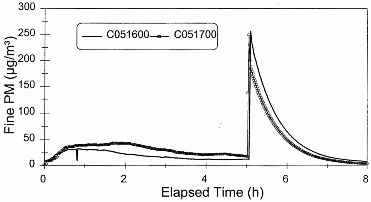
Figure 4. Fine PM concentration profile for candle P2 in test C121699
