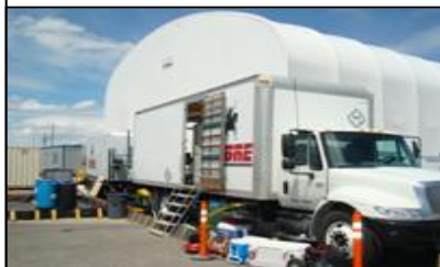
Figure 6. Truck-mounted gas-generation system.
