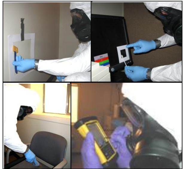
Figure 7. Above: Wipe sampling: sponge-stick and swab. Below: Vacuum sampling (left) and PDA with BROOM software (right).
