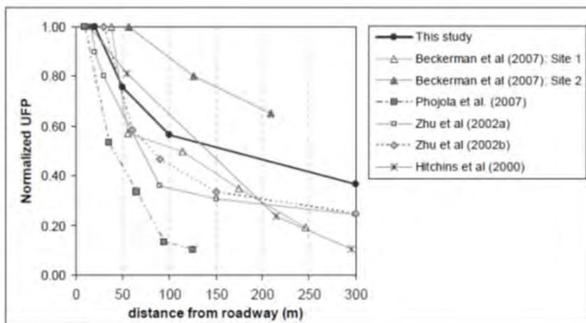
**Figure 1-1.** Ultrafine particles (UFP) as a function of downwind distance from the roadway, with concentrations normalized by the location nearest to the road. Originally published in Hagler et al., (2009).
