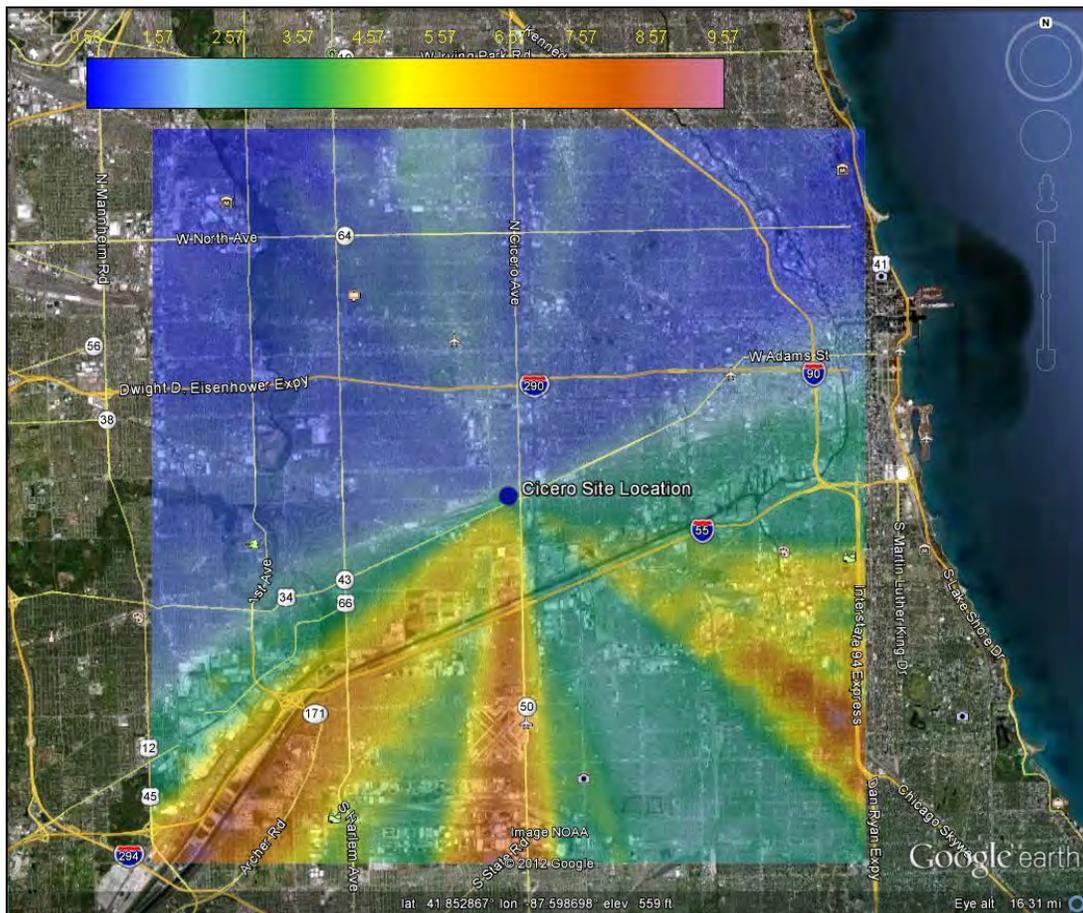
**Figure 3-32.** Sulfur dioxide expected concentration field from NTA.
