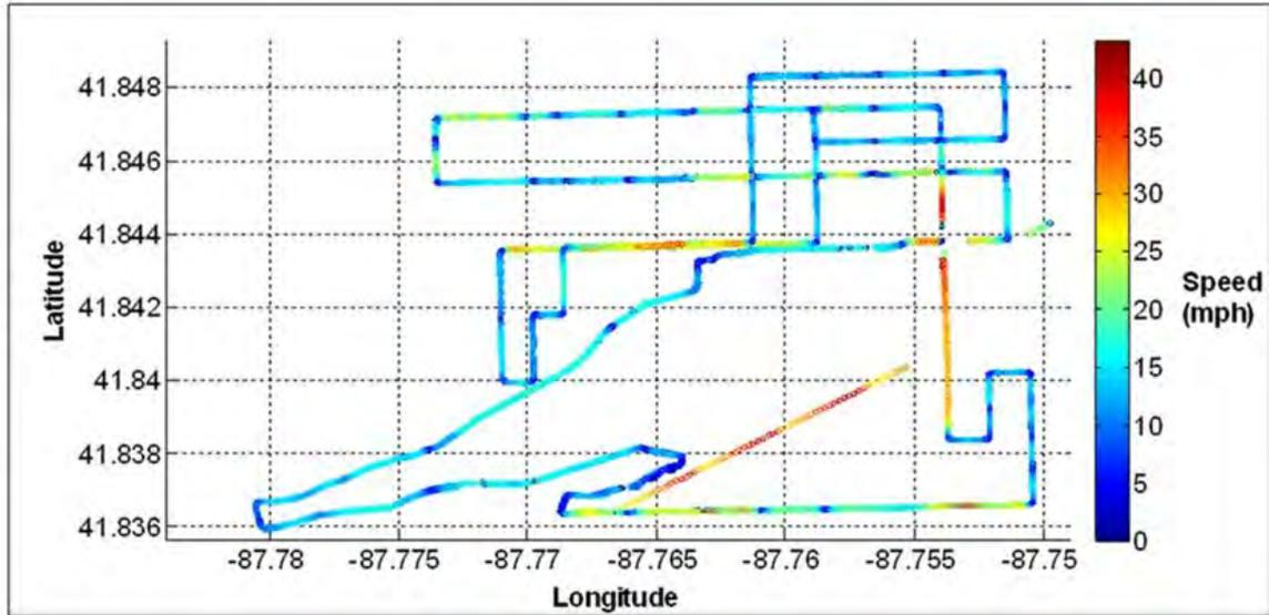
**Figure 3-1.** Driving speed recorded by the sampling vehicle's GPS
