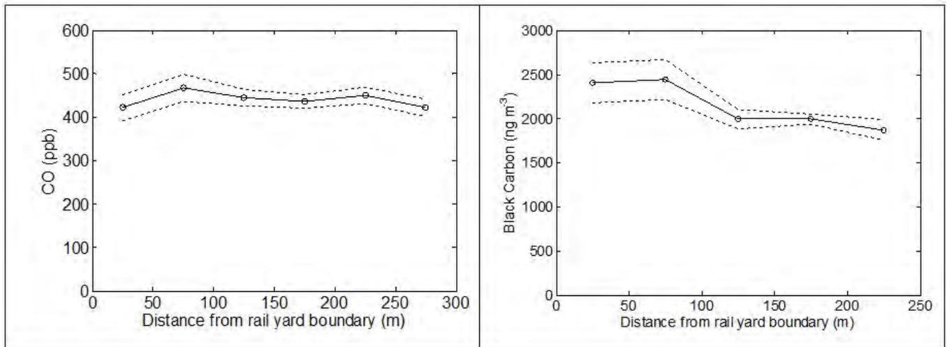
**Figure 2-6.** Example of a concentration versus distance from rail yard boundary figure for CO (left) and black carbon (right). The circle markers indicate the mean value measured and are centered at the midpoint of the distance range; the dashed line indicates the standard error of the measurement.
