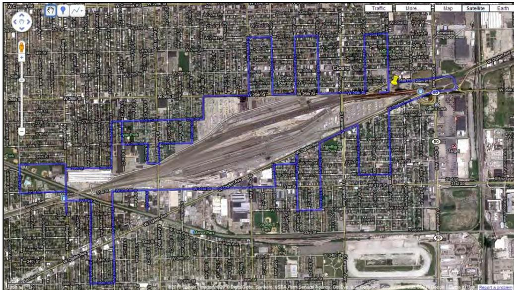
**Figure 5-3.** External rail yard mobile monitoring driving route (blue line) and location for stationary monitoring (yellow marker).
