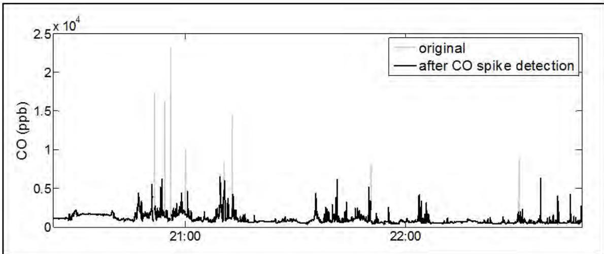
**Figure 2-4.** Example time series of carbon monoxide data, showing the original raw data (gray) and the data time series after detected significant short-term spikes were removed, which were presumably due to local gasoline vehicle exhaust impacting the measurements.
