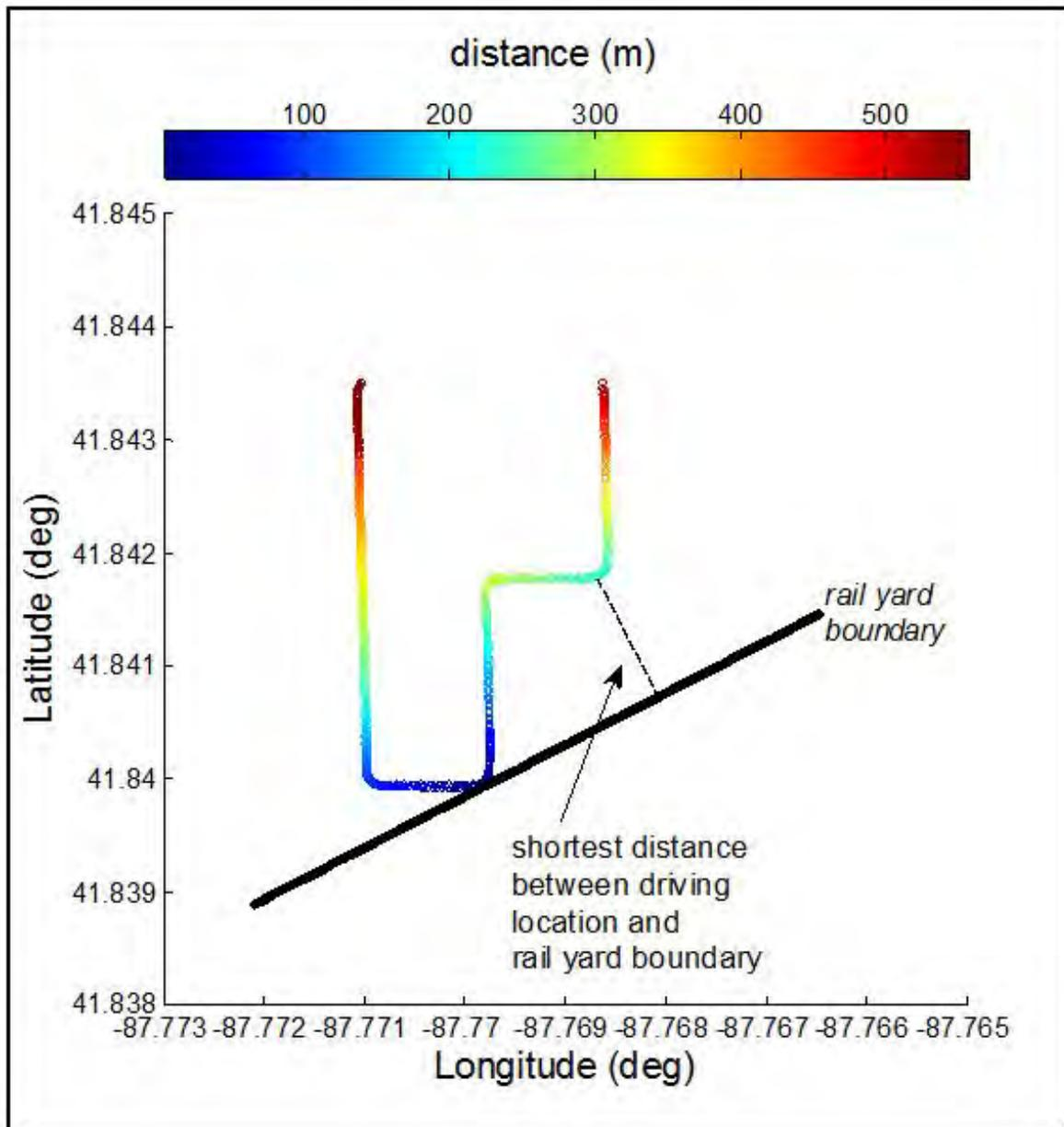
**Figure 2-5.** Example of distance estimated from the pathway driven in neighborhood NT1 relative to the rail yard edge. The dashed line demonstrates the shortest distance from an example location along the driving route to the estimated rail yard boundary line. The shortest distance from each location in neighborhood NT1 to the rail yard boundary is calculated and can be compared to the color bar at the top of the figure.
