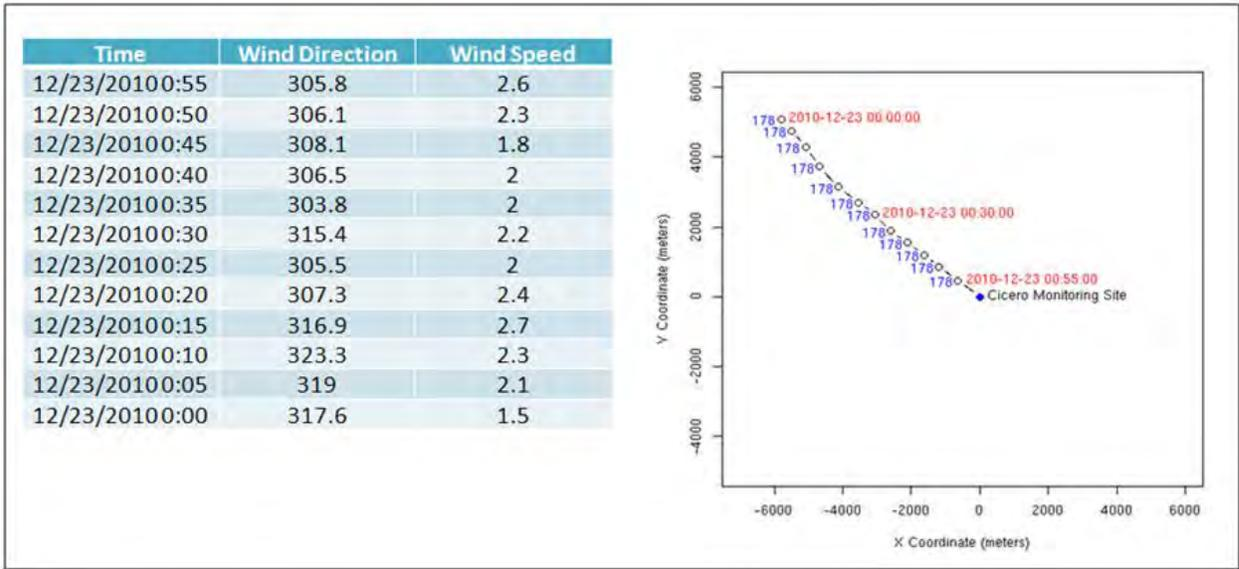
**Figure 2-8.** Example wind data showing how a typical backward trajectory is constructed for NTA. The twelve endpoints making up the hour long trajectory are listed in the table at the left and plotted in the graph. The value of 178 represents a concentration measured at time 2010-12-23 00:55:00.
