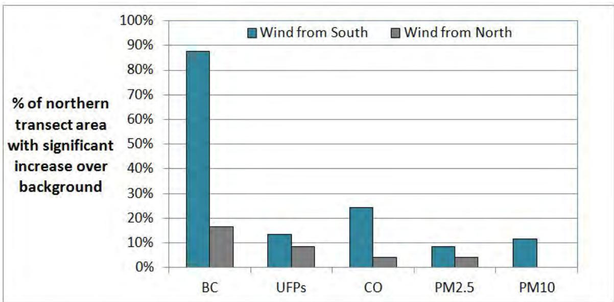
**Figure 3-19.** Fraction of neighborhood areas (NT1-NT4), in 50 m increments up to 300 m from the rail yard, with significant increase in pollutant levels above the background during evening time periods (7-10 PM).
