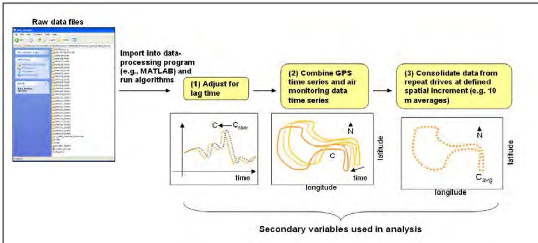
**Figure 9-1.** Post-processing of mobile monitoring raw data for use in analysis.
