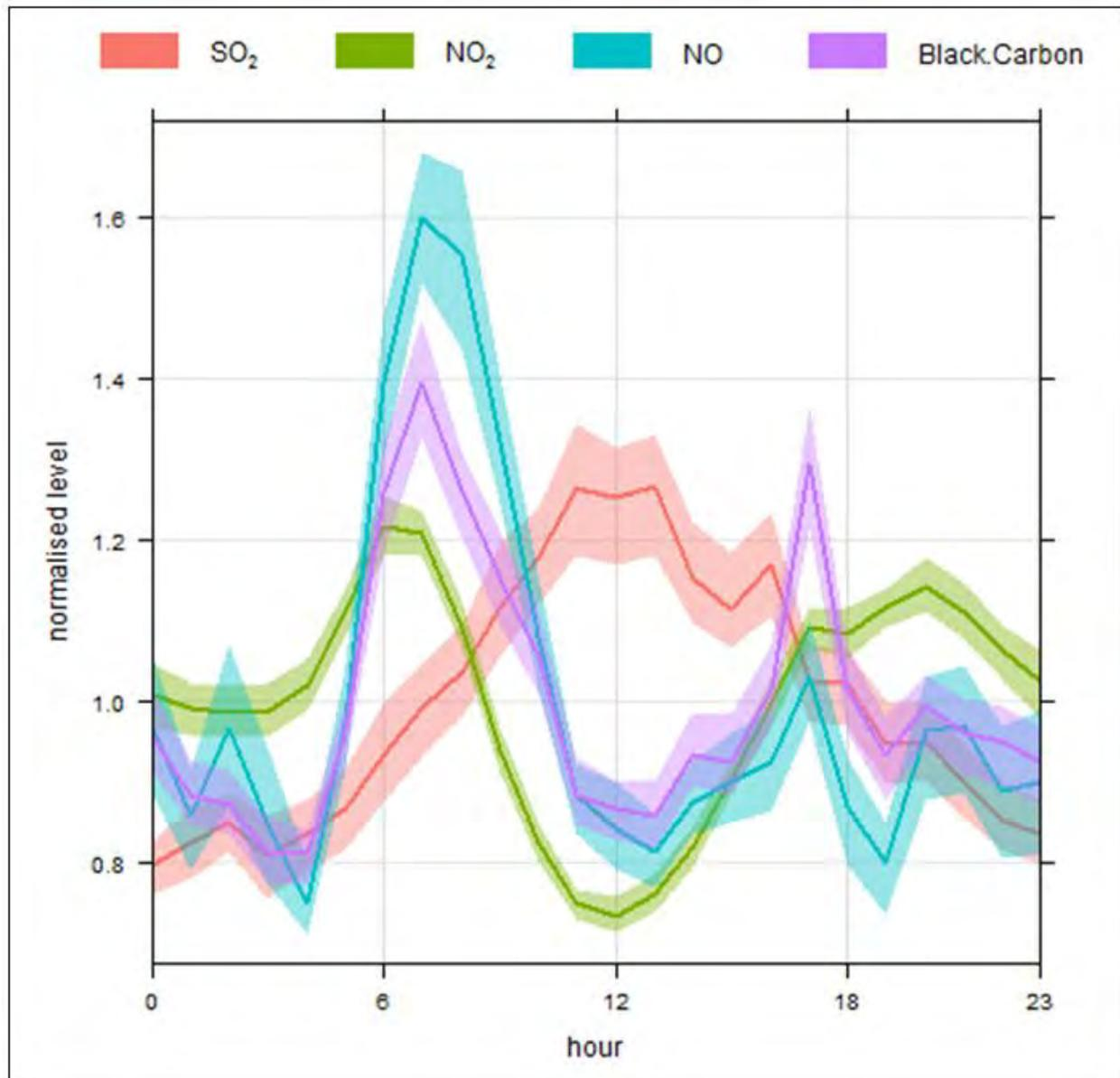
**Figure 3-28.** Normalized diurnal time series of measured concentrations at the stationary monitoring site, for all data collected during November, 2010 – May, 2011.
