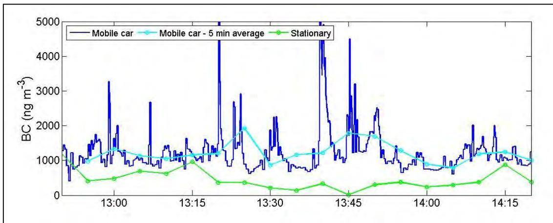
Figure C-3. Intercomparison time series for BC on November 17, 2010, with the y-axis decreased to  $5000 \text{ ng m}^{-3}$  ( $5 \mu\text{g m}^{-3}$ ).
