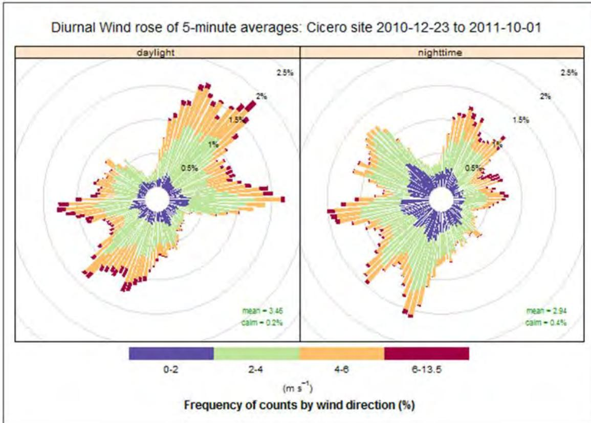
**Figure 3-25.** Cicero stationary monitoring site wind trends during the day (left figure) and night (right figure).
