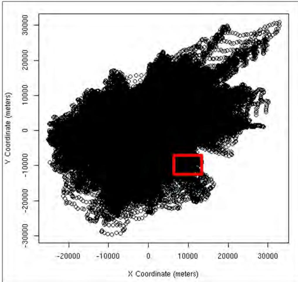
**Figure 2-9.** Example showing all of the backward trajectories for all 5 minute averaged data collected at the Cicero stationary monitor. The red box represents a grid cell for calculating the weighted average at the cell’s center. The cell’s expected concentration would be calculated based on the distance individual trajectory endpoints are from the grid cell’s center.
