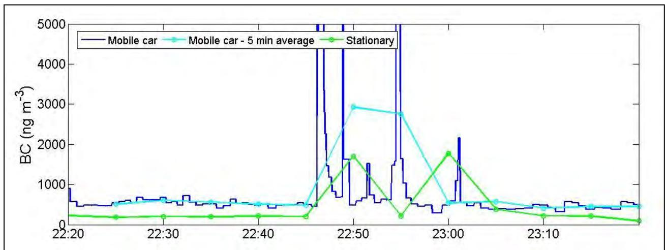
Figure C-8. Intercomparison time series for BC on November 21, 2010, with the y-axis decreased to  $5000 \text{ ng m}^{-3}$  ( $5 \mu\text{g m}^{-3}$ ).
