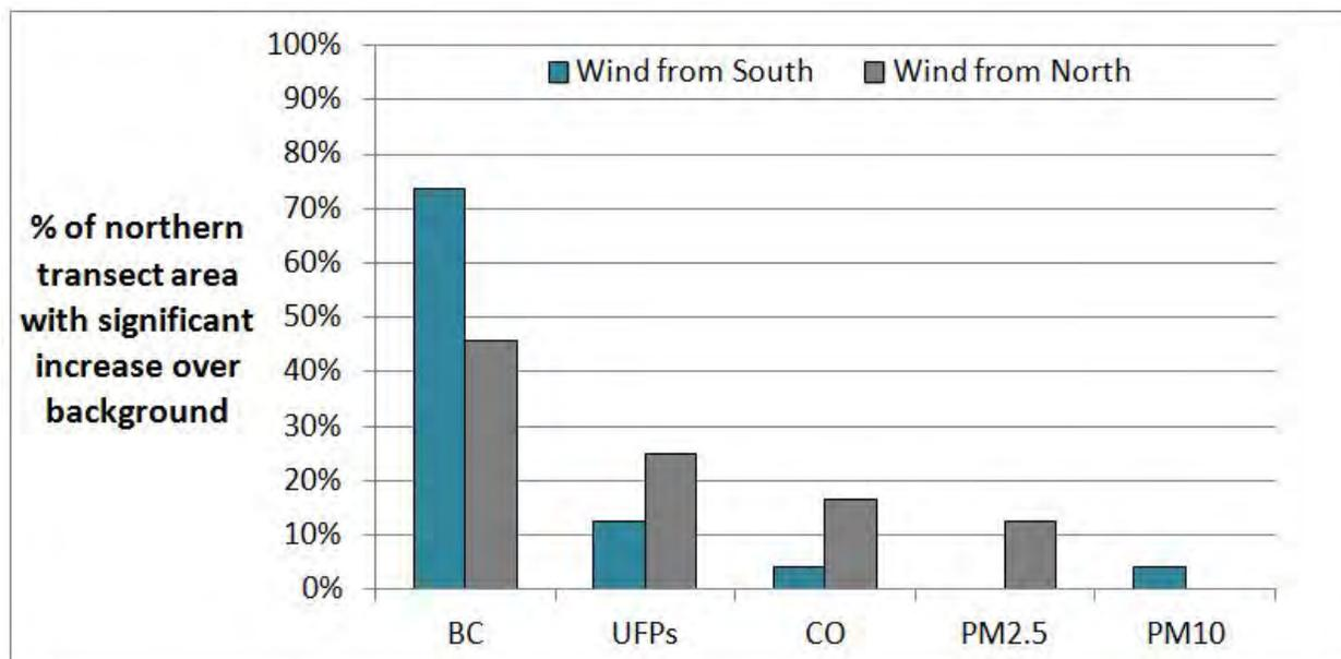
**Figure 3-18.** Fraction of neighborhood areas (NT1-NT4), in 50 m increments up to 300 m from the rail yard, with significant increase in pollutant levels above the background during mid-afternoon time periods (~10 AM-1 PM).
