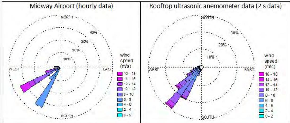
**Figure 3-4.** Comparison of wind measurements collected at Midway airport (left) with wind data collected on top of a BNSF building (right).
