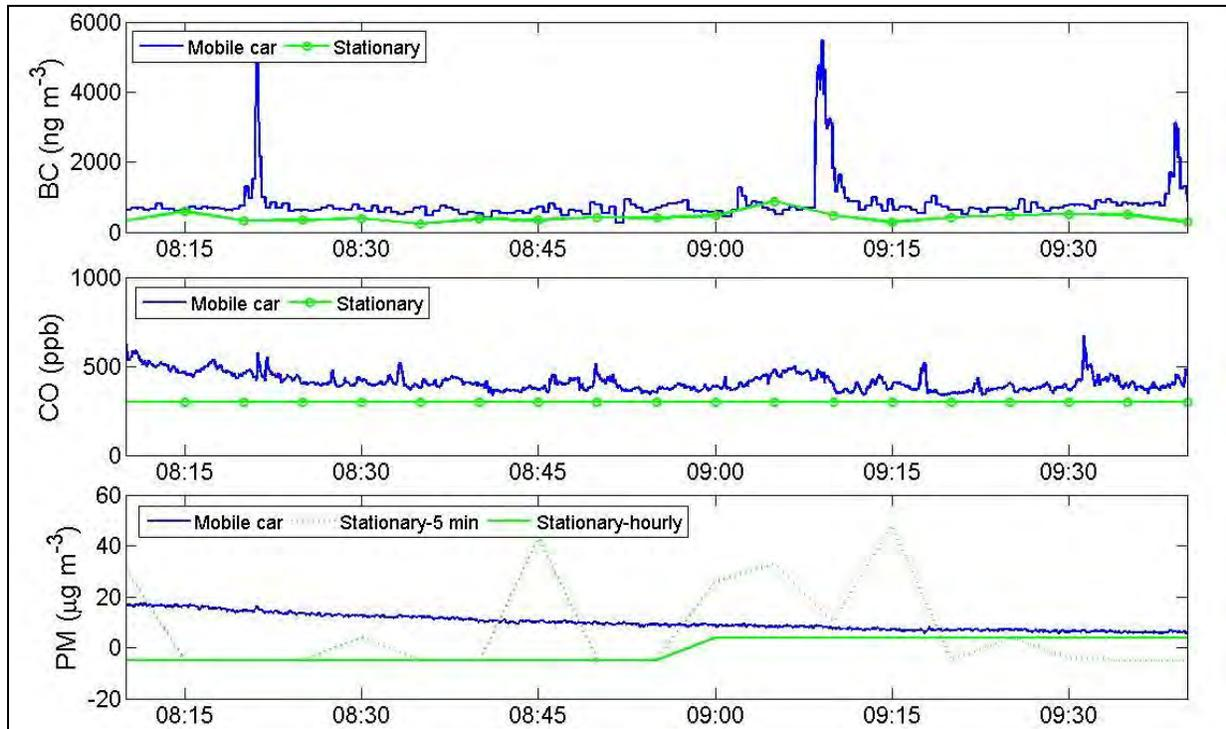
Figure C-7. Intercomparison time series for BC, CO, and  $\text{PM}_{2.5}$  on November 20, 2010.
