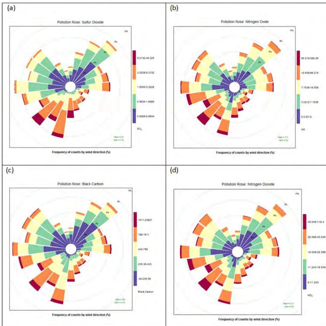
**Figure 3-26.** Concentration roses for sulfur dioxide (ppb) (a), nitrogen oxide (ppb) (b), black carbon ( $\text{ng m}^{-3}$ ) (c), and nitrogen dioxide (ppb) (d). The extent of a given ray indicates the fraction of data associated with a certain wind direction and the rays are colored by concentration range measured from that particular wind sector (color bins are: 0-25<sup>th</sup>, 25-50<sup>th</sup>, 50-75<sup>th</sup>, 75-95<sup>th</sup>, 95-100<sup>th</sup> percentiles).
