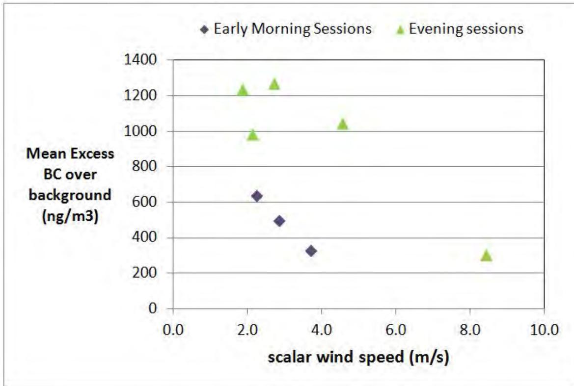
**Figure 3-20.** Mean downwind BC concentrations in neighborhood areas up to 300 m from the rail yard, as a function of local wind speed.
