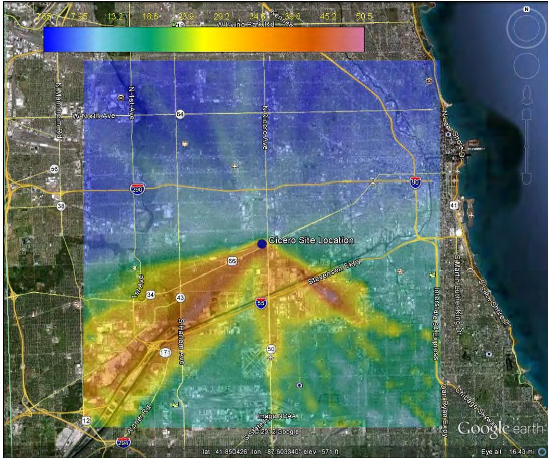
Figure 3-33. Nitric oxide expected concentration field from NTA.
