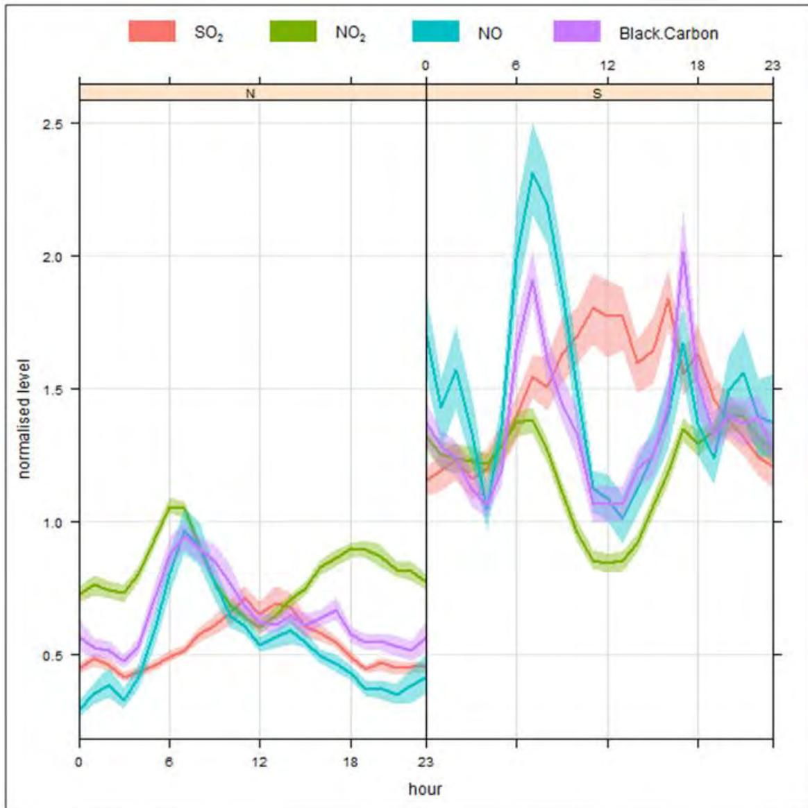
**Figure 3-30.** Normalized diurnal time series of measured concentrations at the stationary monitoring site, for periods of wind from the North (left) and wind from the South (right) collected during November, 2010 – May, 2011.
