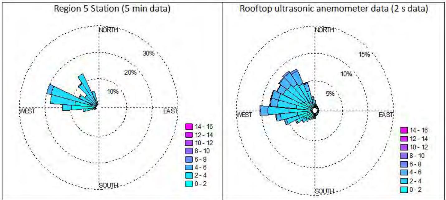
**Figure 3-5.** Comparison of wind measurements collected at the stationary monitoring location (left) with wind data collected on top of a BNSF building (right).
