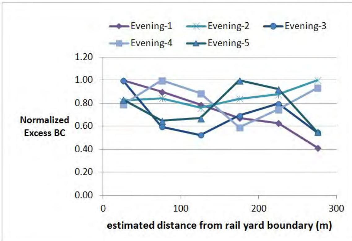
**Figure 3-22.** Normalized downwind excess BC during evening sampling sessions in neighborhood areas up to 300 m from the rail yard, as a function of distance from the rail yard. Concentration markers are located at the midpoint of the distance range (e.g., 25 m for 0-50 m). Points for a given line are normalized by the highest excess BC value for that data series.
