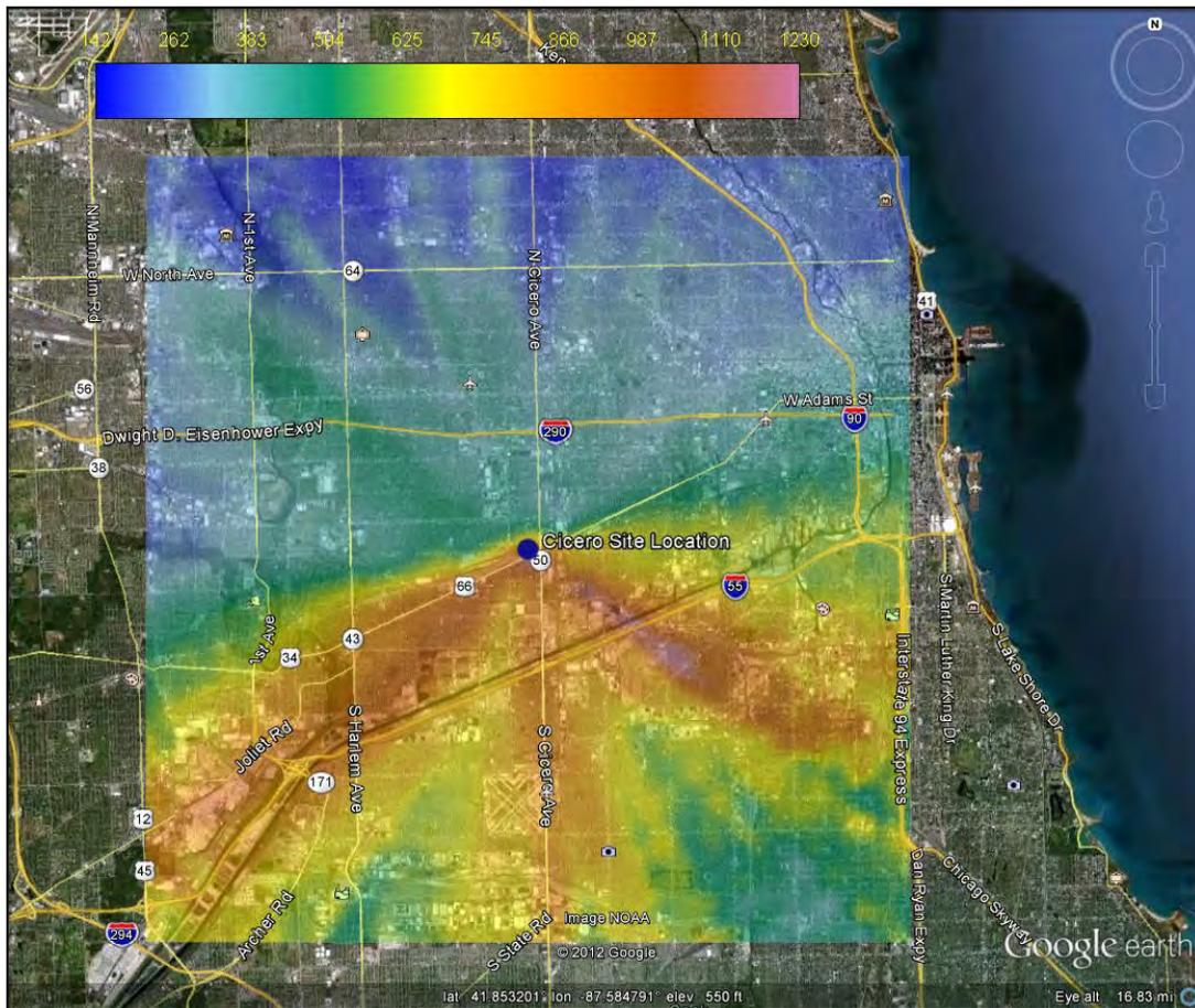
**Figure 3-31.** Black carbon expected concentration field from NTA in  $\text{ng}/\text{m}^3$
