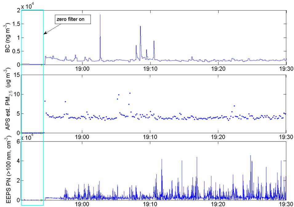
**Figure 3-3.** Example particulate time series during the addition of a zero filter and after the filter is removed. The filter-on period is marked with the light blue box.
