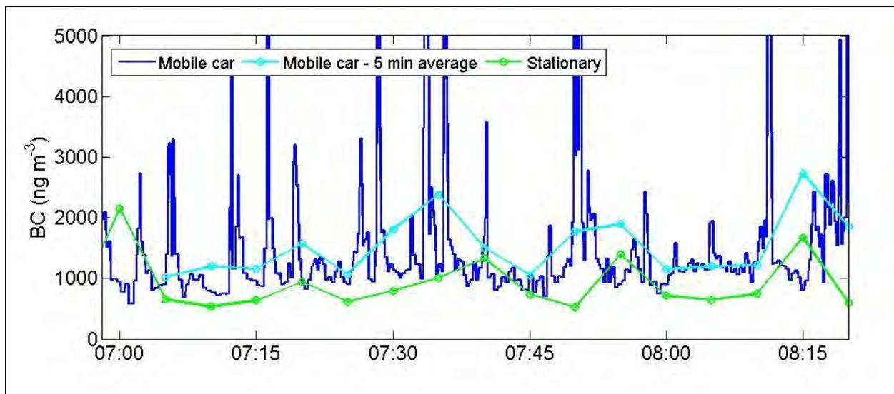
Figure C-6. Intercomparison time series for BC on November 19, 2010, with the y-axis decreased to  $5000 \text{ ng m}^{-3}$  ( $5 \mu\text{g m}^{-3}$ ).
