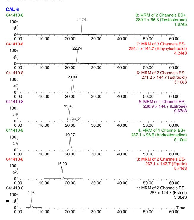
FIGURE 2. EXAMPLE CHROMATOGRAM OF LC-ESI-MS/MS TRANSITIONS FOR METHOD 539 SURROGATES AND INTERNAL STANDARDS.
