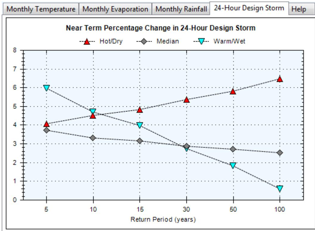
**Figure 4 Example of 24-Hour Design Storm Adjustments**
