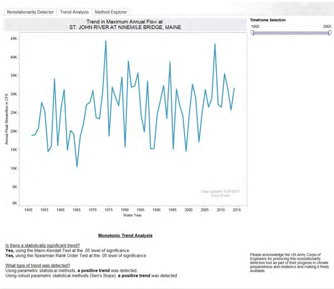
Figure 3: USACE Nonstationarity Detection Tool trend analysis screenshot
