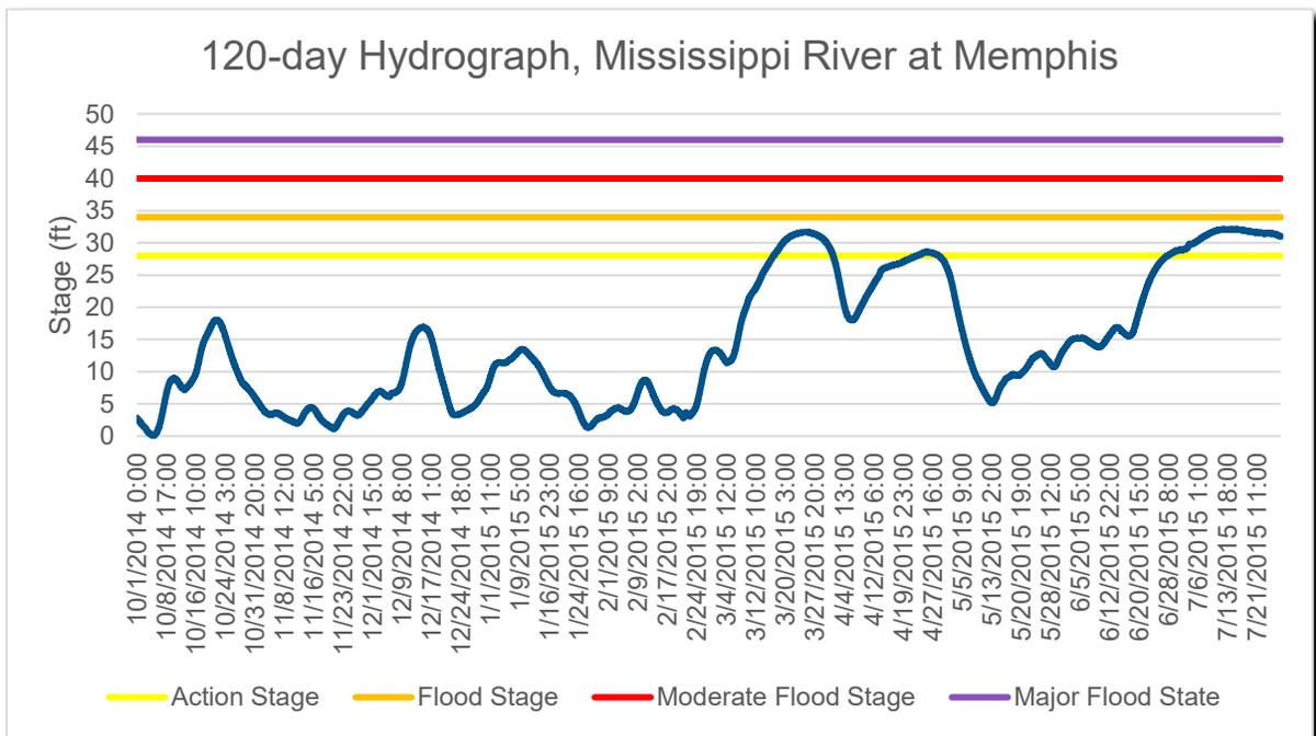
Figure 6: Example hourly river levels (shown for the 120-day period, 10/1/2014–7/21/2015) (chart developed by ICF using data from USGS National Water Information System, Mississippi River at Memphis)
