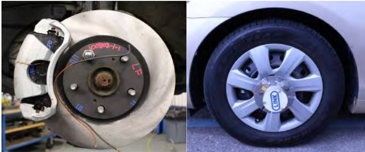
Figure 4. Brake Thermocouples and wireless hub transmitter installed on the Camry test vehicle
