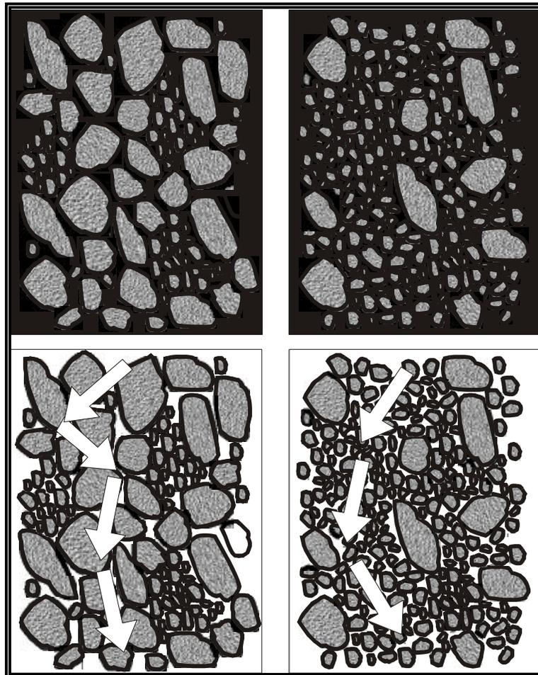
**Figure 2.3.** Schematic diagram for conceptual model of water distribution in saturated (top two figures) and unsaturated soils (bottom two figures) suggesting differences in the unsaturated flow regime (indicated by arrows) for soils with varying texture. [The two figures on left represent coarse-textured soils, whereas the two figures on the right represent fine-textured soils. Soil particles, air, and water are shown, respectively, in stippled gray, white, and black.]
