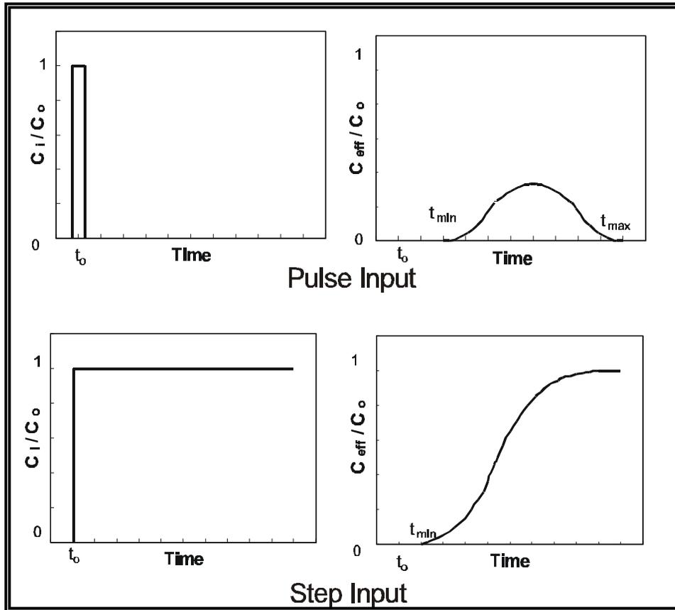
**Figure 3.4.** Schematic diagram showing the relative concentrations of a constituent at the input source (figures on left) and in the effluent (figures on right) as a function of time for a pulse versus step input. [ $C_o$ ,  $C_i$ , and  $C_{eff}$  refer, respectively, to the concentration of the constituent at  $t_0$  and the concentrations of the constituents in the input and effluent.]
