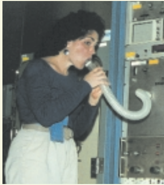
A volunteer in an ozone research study breathes into a spirometer—a device that measures lung function.
