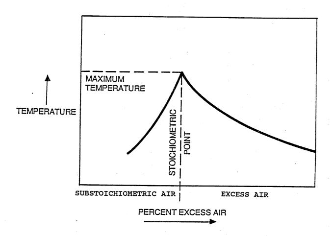
Figure 10. Relationship between temperature and combustion air levels.
