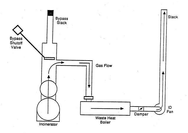
Figure 11. MWI with a waste heat recovery boiler and bypass stack.
