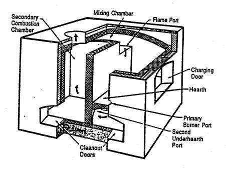
Figure 7. Retort hearth incinerator.
