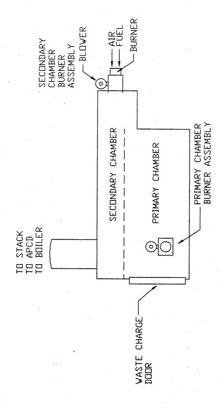
Schematic of a single batch-duty medical waste incinerator. Figure 6.
