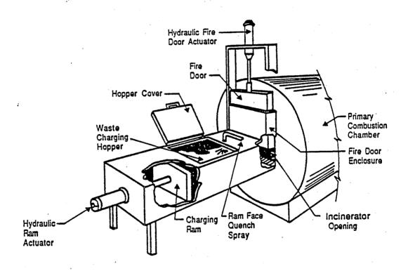
Figure 8. Hopper/ram mechanical waste feed system.  $^{25}$
