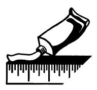
You must check for water in the bottom of the tank at least once each month by smearing a water-finding paste along the bottom of the gauge stick. The paste changes color when it comes in contact with water. Many operators improve their stick readings by smearing a fuel-finding paste on about 6 inches of the stick where they expect the fuel level to be. Fuel-finding paste changes color when it comes in contact with fuel.
